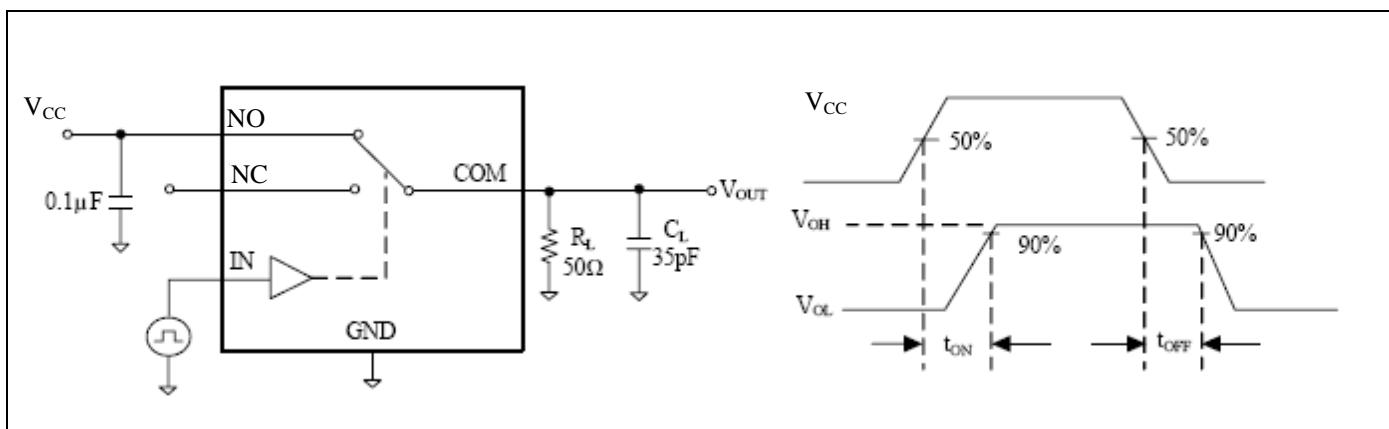
Figure 2. Switching Times
