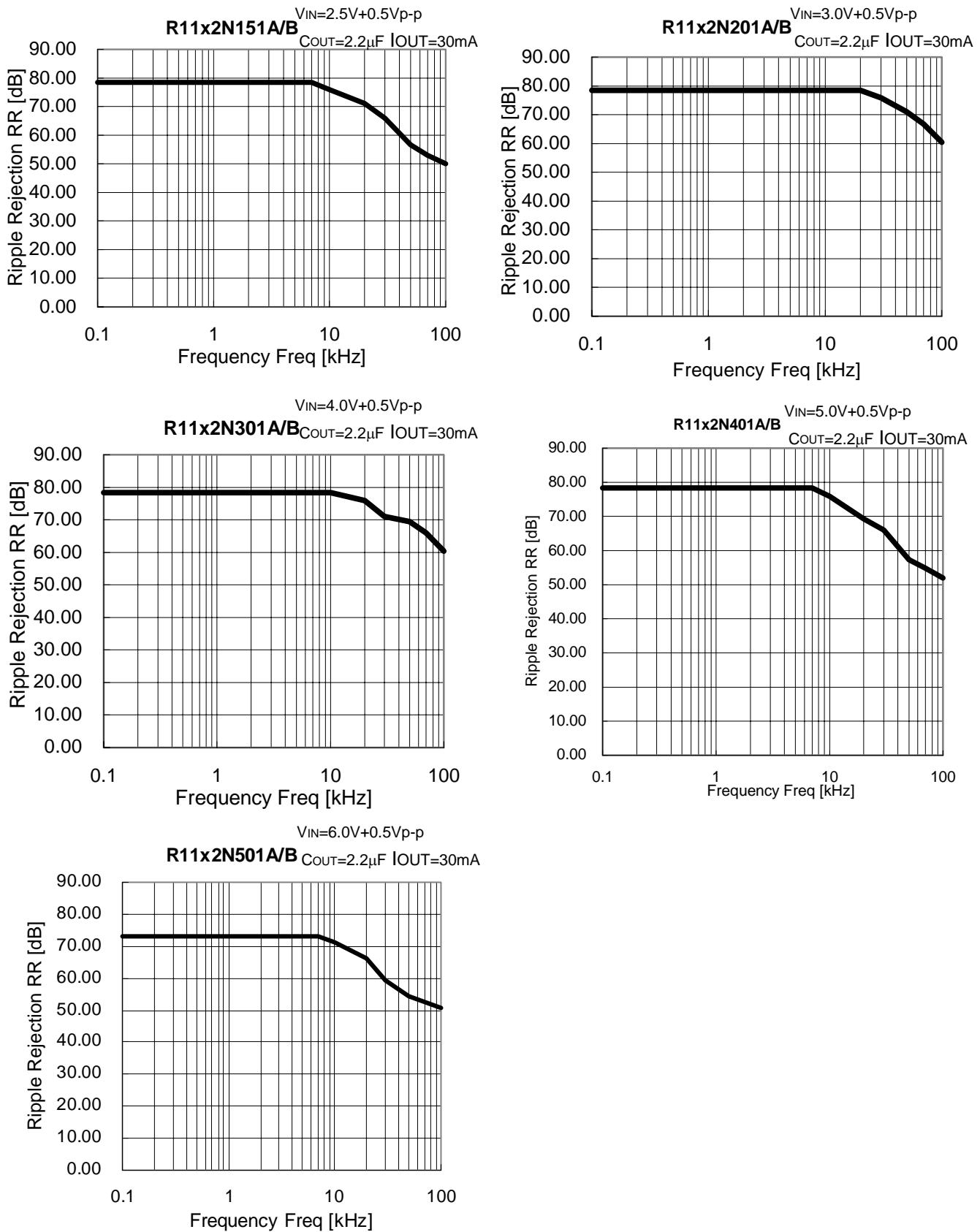
8) Ripple Rejection vs. Input Voltage (DC bias)
