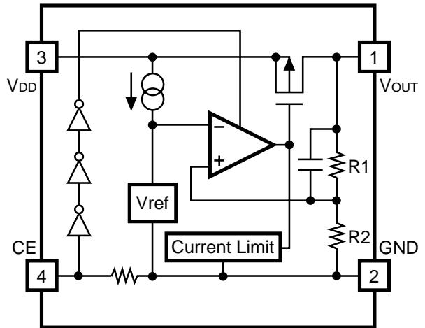
In these ICs, fluctuation of Output Voltage,  $V_{OUT}$  is detected by Feed-back Registers,  $R_1$  and  $R_2$ , and the result is compared with a reference voltage by Error Amplifier, so that a constant voltage is output.
