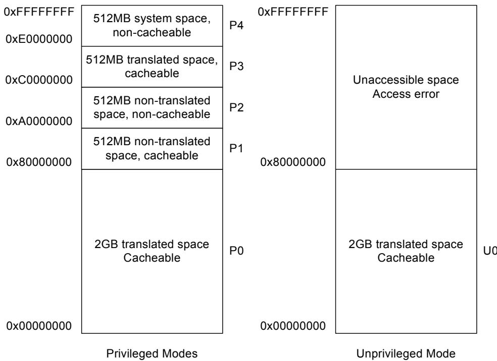
The memory map has six different segments, named P0 through P4, and U0. The P-segments are accessible in the privileged modes, while the U-segment is accessible in the unprivileged mode.
