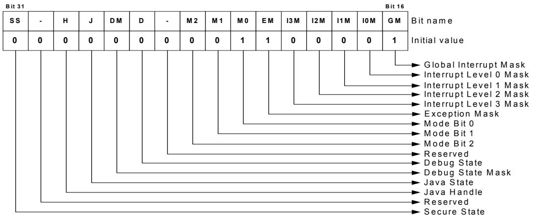
**Figure 2-7.** The Status Register low halfword
