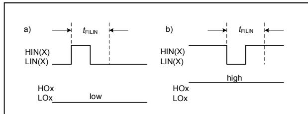
**Figure 4** Input filter timing diagram
