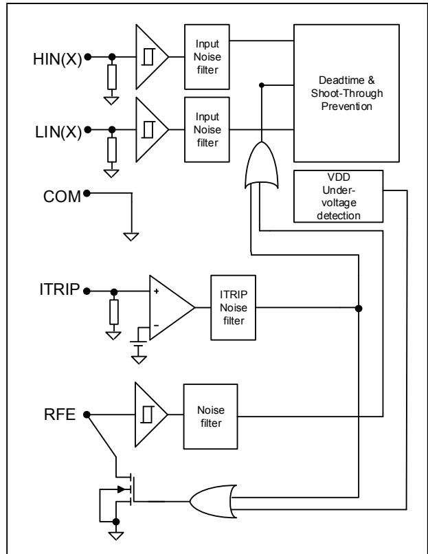
**Figure 6      RFE internal circuit structure**
