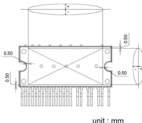
**Figure 8 Backside curvature measurement position**
