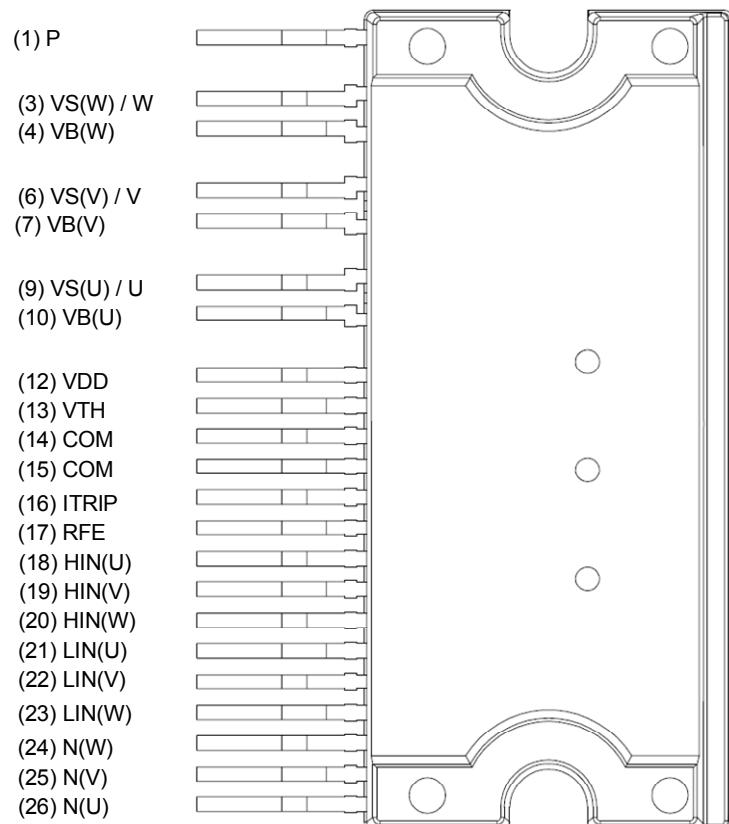
**Figure 2** Pin configuration
