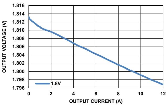
FIGURE 13.  $V_{OUT}$  REGULATION vs LOAD ( $V_{IN} = 12V$ , CCM, 600kHz)
