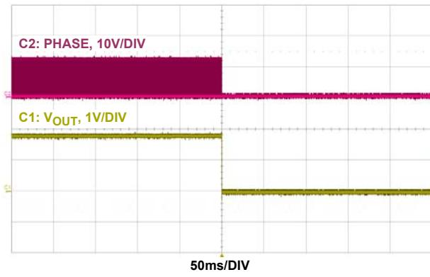
FIGURE 15. LATCH-OFF OCP ( $V_{IN} = 12V$ ,  $V_{OUT} = 1.8V$ , 600kHz, CCM)
