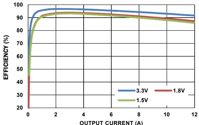
FIGURE 12. EFFICIENCY vs LOAD ( $V_{IN} = 5V$ , CCM, 600kHz)
