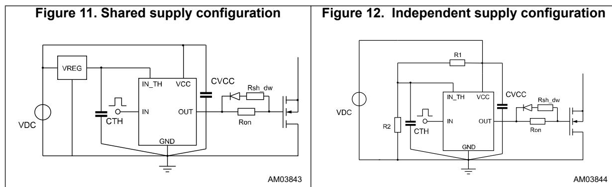
It is mandatory to properly connect a 100 nF ceramic cap as close as possible to the VCC pin to bypass the current's spikes absorbed by VCC during the gate charging.
