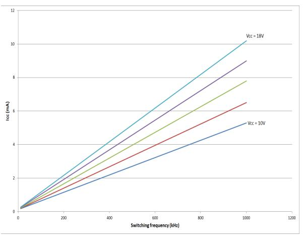
**Figure 6.  $V_{CC}$  power dissipation (PD) when no load is applied**
