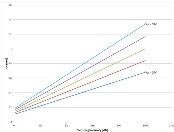
**Figure 5. Operating supply current ( $C_{OUT} = 470 \text{ pF}$ )**
