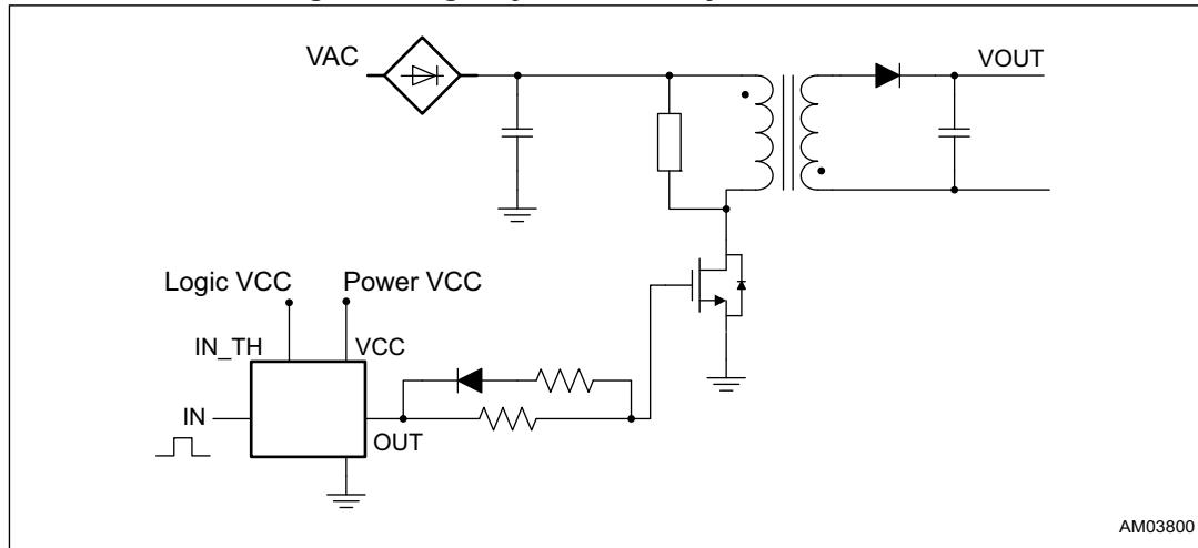
**Figure 10. Digitally controlled inverse buck converter (e.g.: LED controller)**
