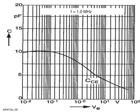
Figure 6. Transistor Capacitance (typ.) vs. Collector-Emitter Voltage
