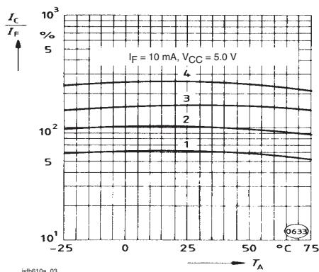
Figure 3. Current Transfer Ratio (CTR) vs. Temperature
