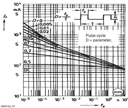
Figure 7. Permissible Pulse Handling Capability Forward Current
