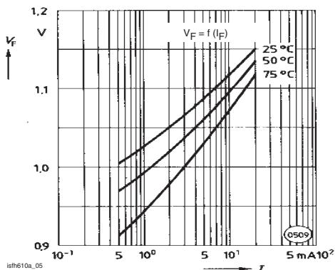
Figure 5. Diode Forward Voltage vs. Forward Current
