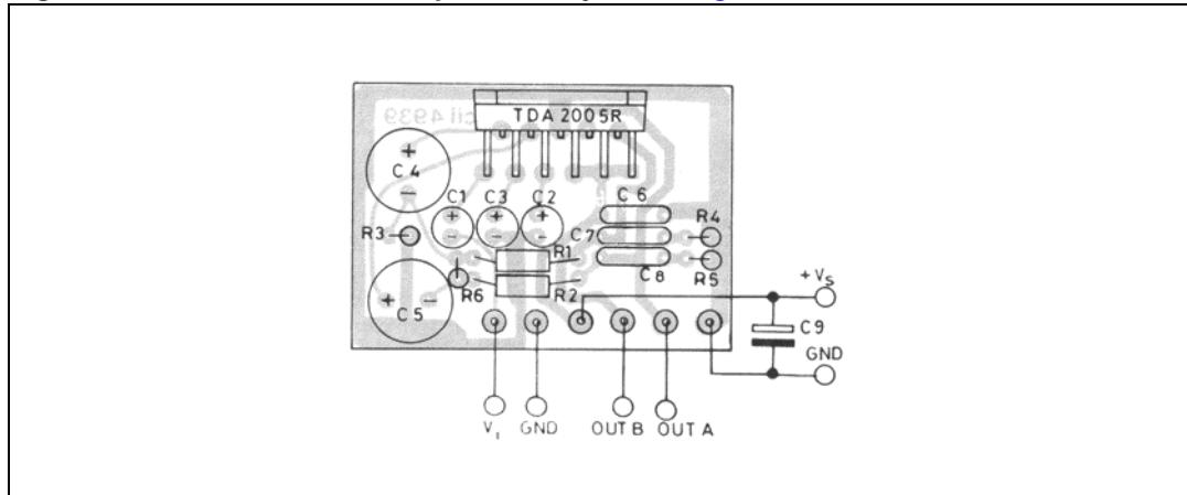
**Figure 27. Low cost bridge amplifier ( $G_V = 42 \text{ dB}$ )**
