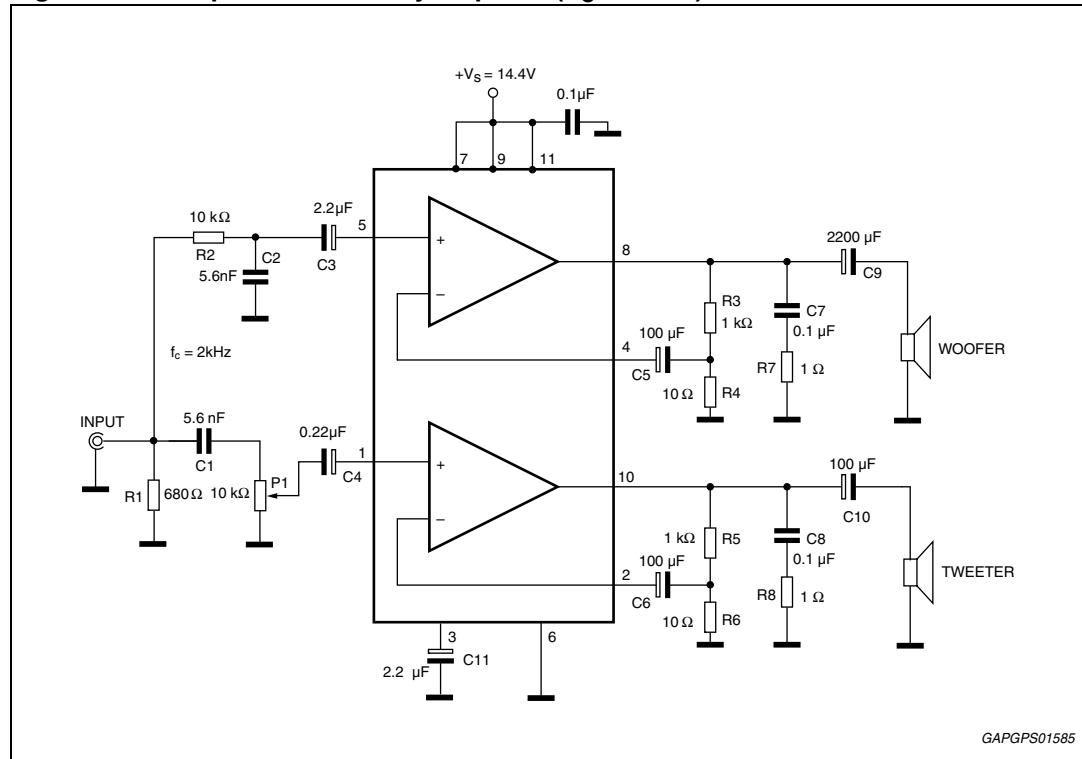
**Figure 33.** Bridge amplifier circuit suited for low-gain applications ( $G_V = 34 \text{ dB}$ )
