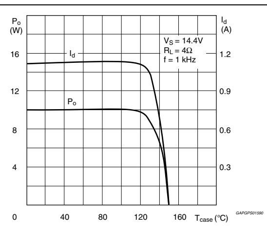
**Figure 39. Output power and drain current vs. case temperature ( $R_L = 3.2 \Omega$ )**
