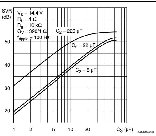
**Figure 20. Supply voltage rejection vs. C<sub>2</sub> and C<sub>3</sub>, G<sub>V</sub> = 1000/10 Ω (stereo amplifier)**
