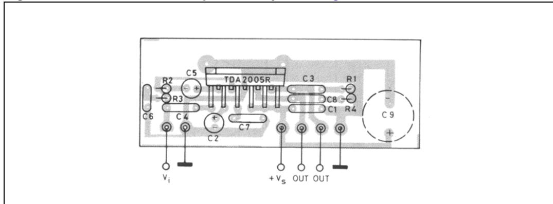
**Figure 29.** 10 + 10 W stereo amplifier with tone balance and loudness control
