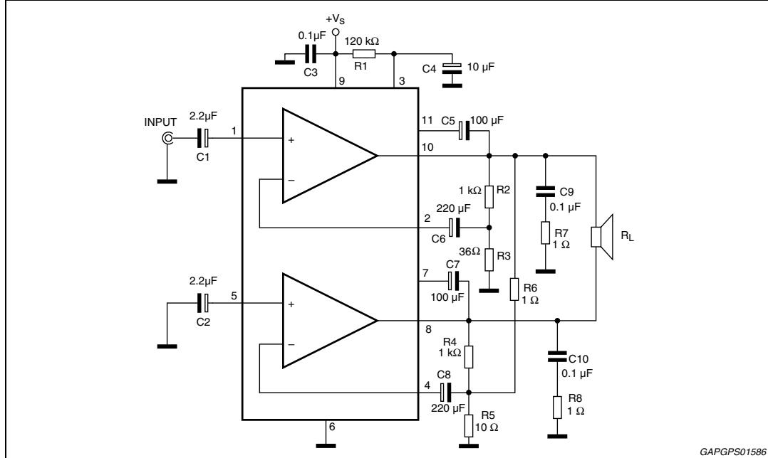
**Figure 34.** Example of muting circuit
