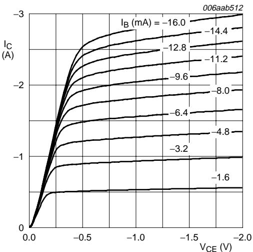
**Fig 6.** TR1 (PNP): Collector current as a function of collector-emitter voltage; typical values
