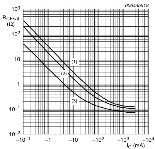
**Fig 12.** TR1 (PNP): Collector-emitter saturation resistance as a function of collector current; typical values
