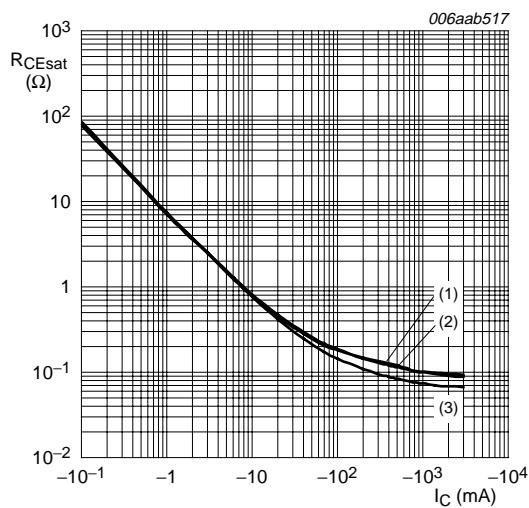
**Fig 11.** TR1 (PNP): Collector-emitter saturation resistance as a function of collector current; typical values
