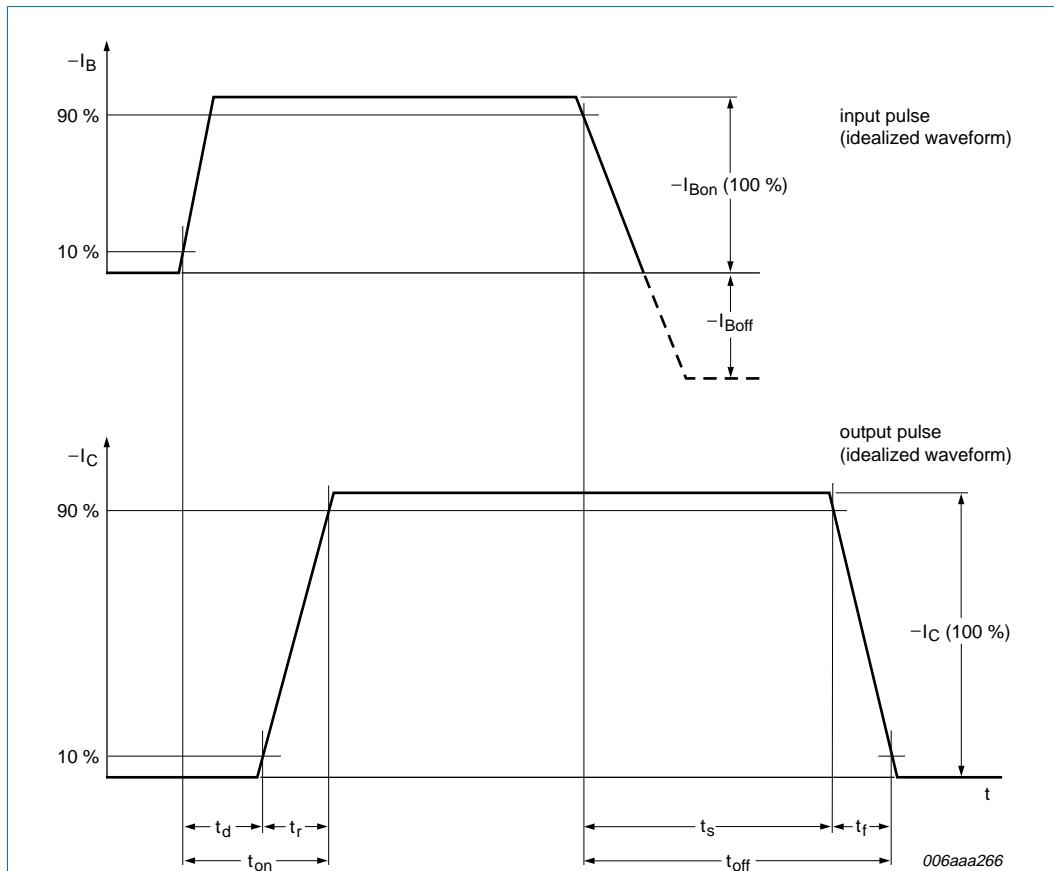
**Fig 18. TR1: BIAS transistor switching time definition**
