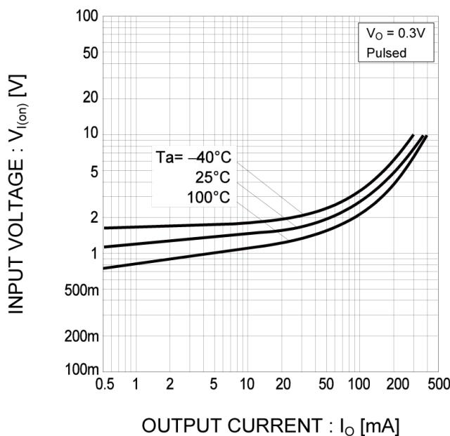
Fig.2 Output Current vs. Input Voltage
