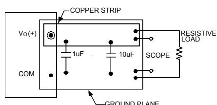
Figure 44. Output Ripple and Noise Test Setup.
