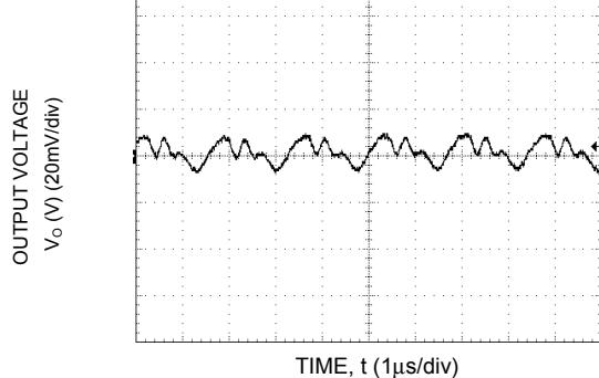
Figure 3. Typical output ripple and noise ( $V_{IN} = 9V$ ,  $I_o = I_{o,max}$ ).
