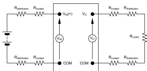
Figure 45. Output Voltage and Efficiency Test Setup.
