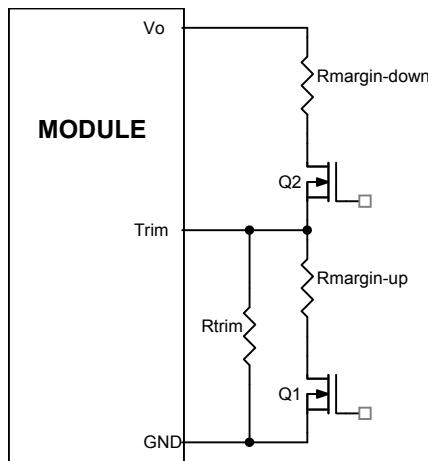
Figure 51. Circuit Configuration for margining Output voltage.
