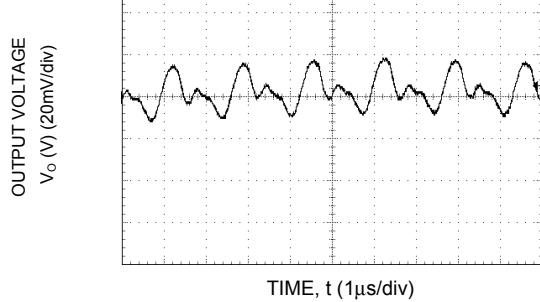
Figure 15. Typical output ripple and noise ( $V_{IN} = 12V$ ,  $I_o = I_{o,max}$ ).
