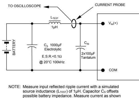
Figure 43. Input Reflected Ripple Current Test Setup.
