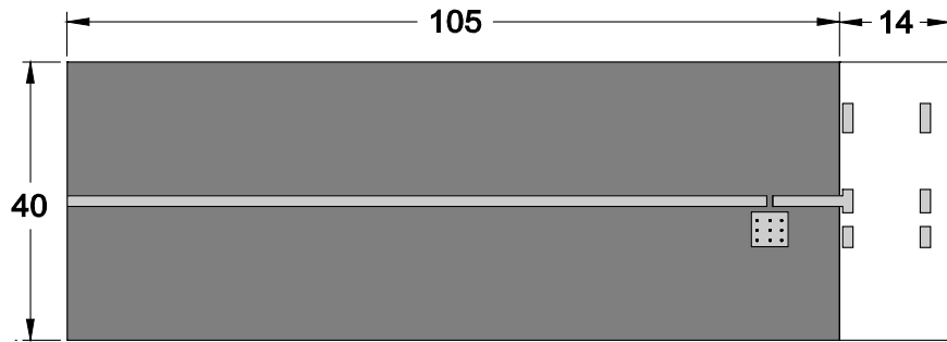
Fig. 2 Outlook and dimension of evaluation board
