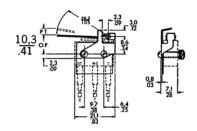
Figure 2. MICRO SWITCH™ HM, Wire Leads
