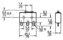
MOUNTING HOLES WILL ACCEPT PINS OR SCREWS OF 1,9/.08 DIA
