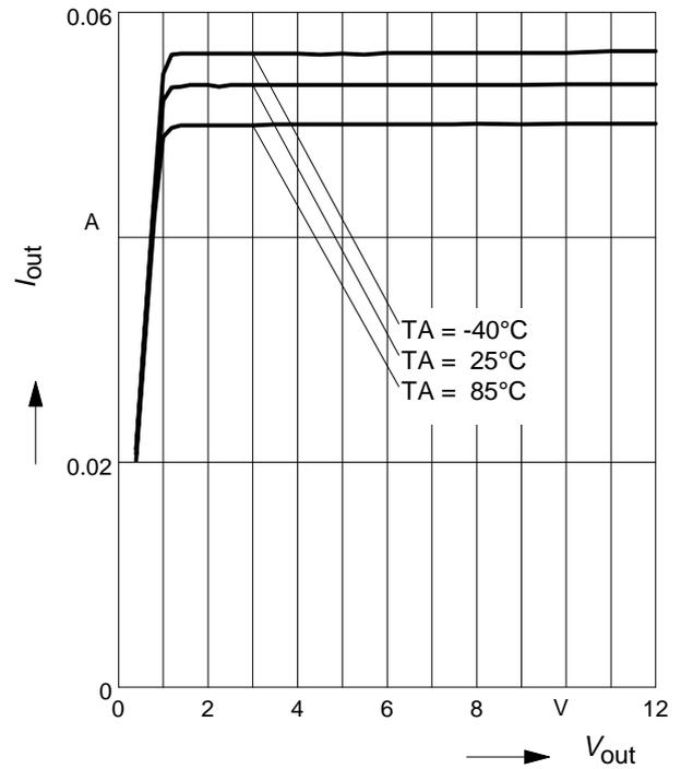
**BCR421U: Output current versus  $V_{out}$**
