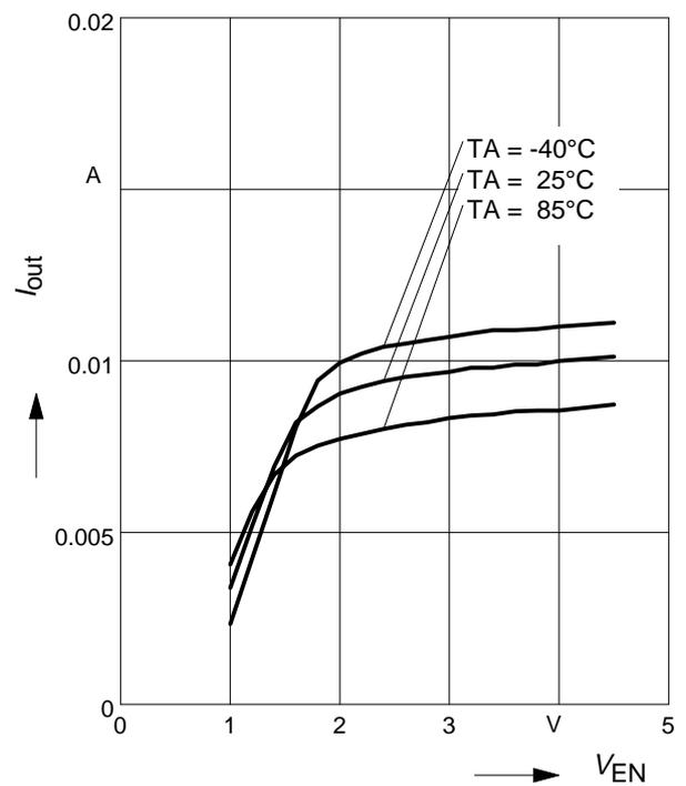
**BCR421U: Output current versus  $V_{EN}$**
