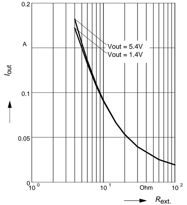
**BCR420U: Output current versus  $V_{out}$**
