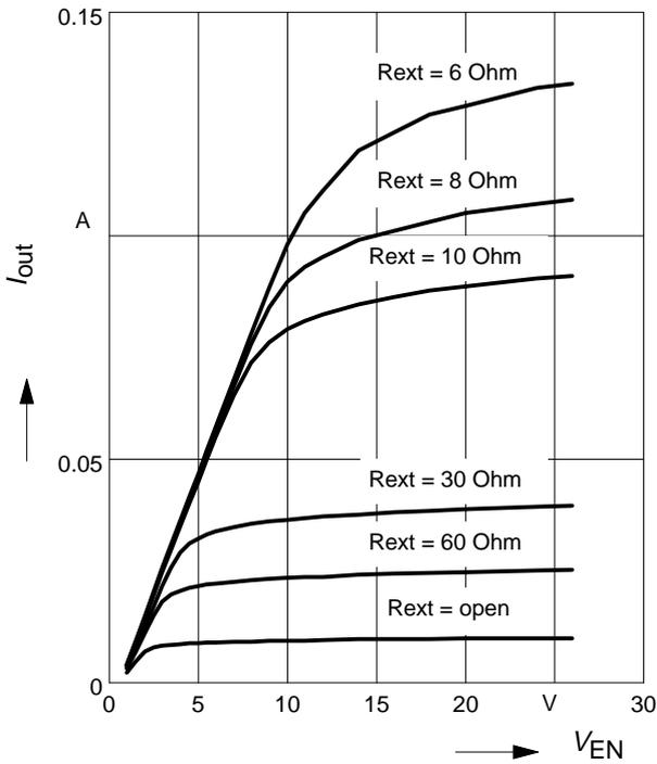
**BCR420U: Enable current versus  $V_{EN}$**
