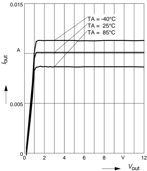
**BCR320U: Output current versus  $V_{out}$**
