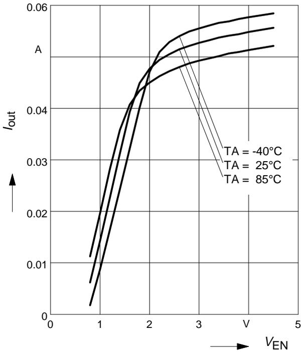
**BCR421U: Output current versus  $V_{EN}$**
