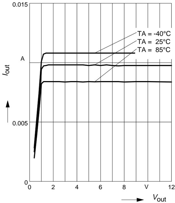
**BCR421U: Output current versus  $V_{out}$**
