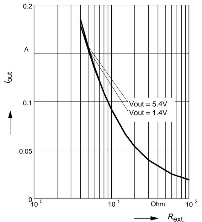
**BCR421U: Output current versus  $V_{out}$**
