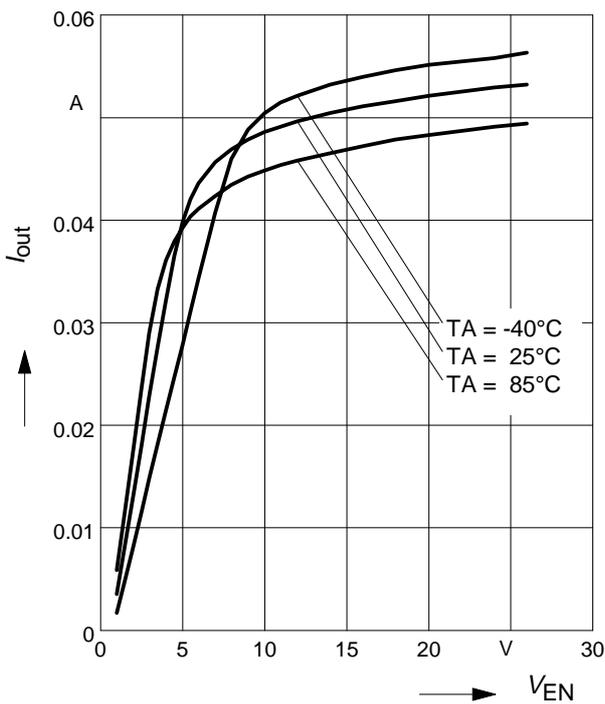
**BCR420U: Output current versus  $V_{EN}$**
