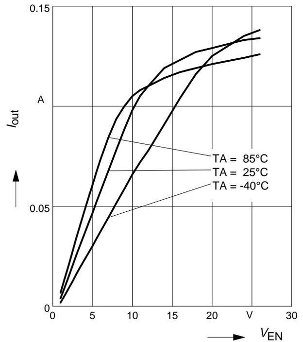
**BCR420U: Output current versus  $V_{EN}$**
