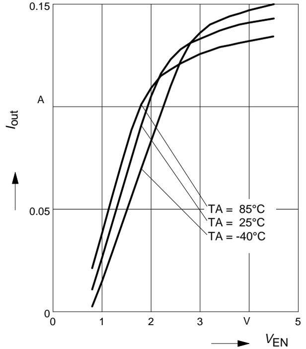
**BCR421U: Output current versus  $V_{EN}$**
