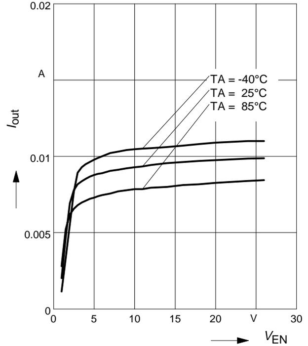
**BCR420U: Output current versus  $V_{EN}$**
