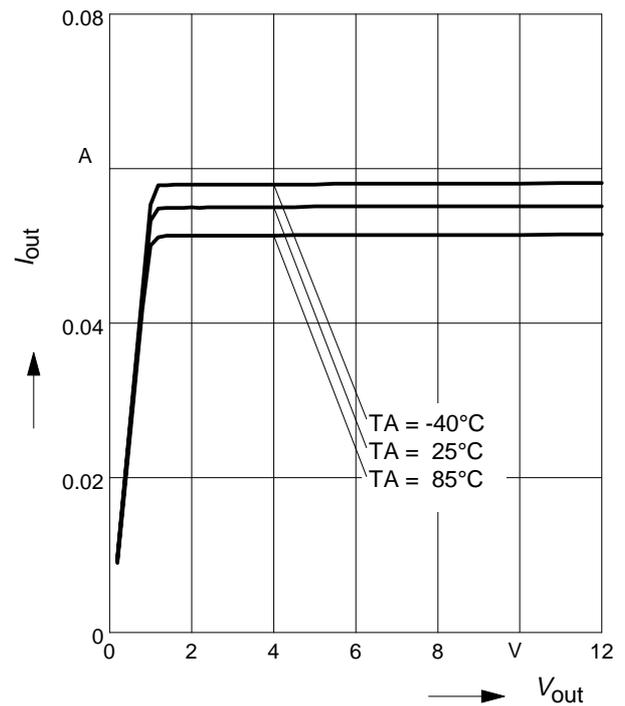
**BCR420U: Output current versus  $V_{out}$**
