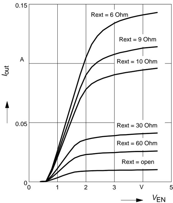
**BCR421U: Enable current versus  $V_{EN}$**
