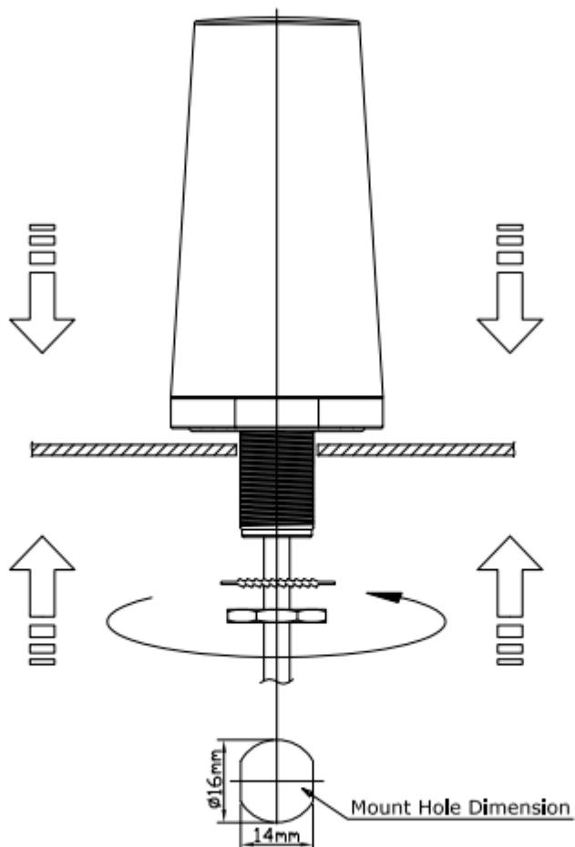
Recommended torque for mounting is 4.018 N.m or 41 kgf.cm
