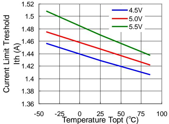
**11) Current Limit Threshold vs. Input Voltage
