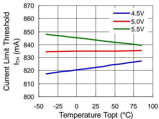
**10) Current Limit Threshold vs. Temperature
