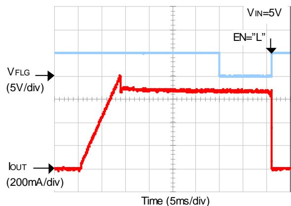
**21) Overcurrent Response with Ramped Load****(R5524x004A)**
