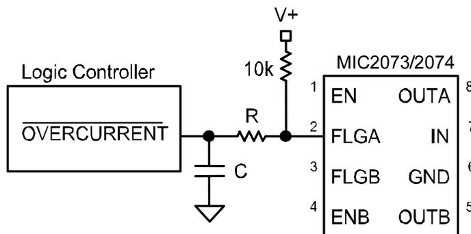
Figure 4. Transient Filter
