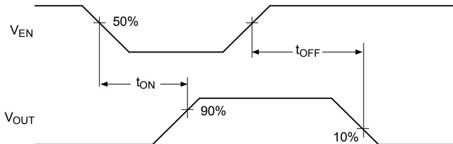
Active-Low Switch Delay Times (MIC2073-2/2074-2)
