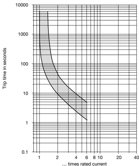
The time/current characteristic curve depends on the ambient temperature prevailing. In order to eliminate nuisance tripping, please multiply the circuit breaker current ratings by the derating factor shown below. See also section Technical information.
