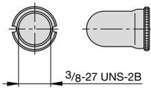
Hex nut with splash cover black without O ring X 210 739 01 (IP64) transparent splash cover X 201 296 03 (IP64)
