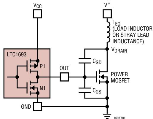
Figure 1. Capacitance Seen by OUT During Switching
