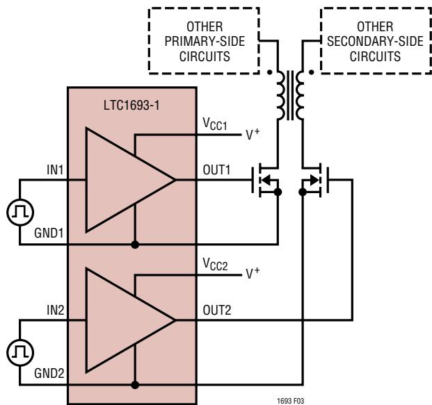
Figure 3. Simplified LTC1693-1 Application with Different Ground Potentials
