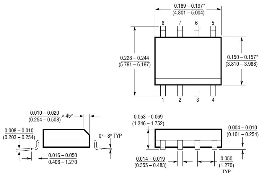
\*DIMENSION DOES NOT INCLUDE MOLD FLASH. MOLD FLASH
