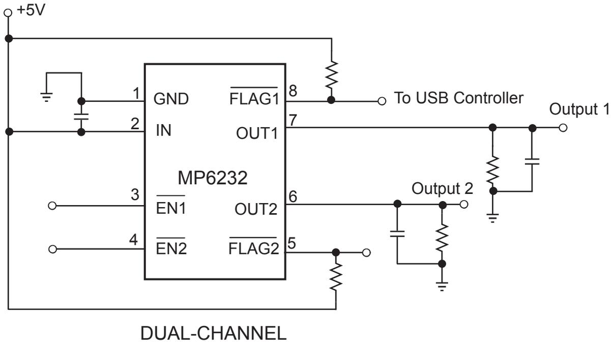
Figure 3—Application Circuit
