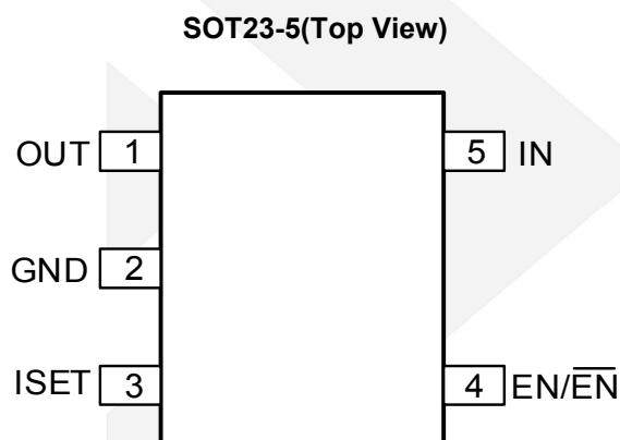
Figure 1 Pin Assignment
