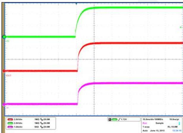
**V<sub>IN</sub> Shut down (R<sub>OUT</sub>=2.5Ω)**
