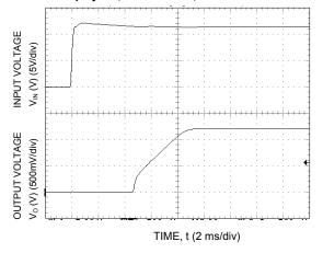
Figure 12. Typical Start-up Using Input Voltage (VIN = 12V,  $I_0 = I_{0,max}$ ).
