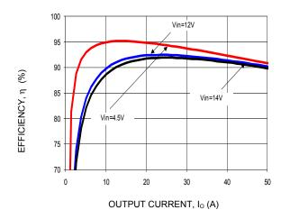
Figure 13. Converter Efficiency versus Output Current.
