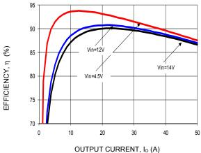
Figure 7. Converter Efficiency versus Output Current.
