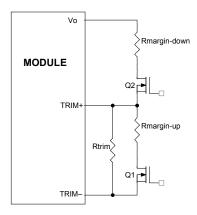
Figure 26. Circuit Configuration for margining Output voltage.
