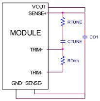
Figure. 28. Circuit diagram showing connection of  $R_{\text{TUME}}$  and  $C_{\text{TUNE}}$  to tune the control loop of the module.
