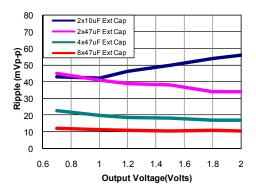
Figure 23. Output ripple voltage for various output voltages with external 2x10  $\mu$ F, 2x47  $\mu$ F, 4x47  $\mu$ F or 8x47  $\mu$ F ceramic capacitors at the output (50A load). Input voltage is 12V.
