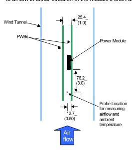
Figure 29. Thermal Test Setup.
