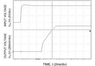
Figure 5. Typical Start-up Using On/Off Voltage ( $I_0 = I_{0,max}$ ).
