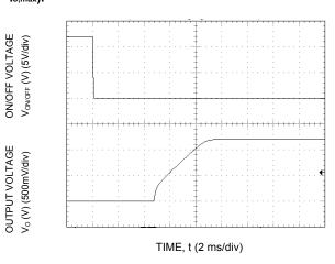
Figure 11. Typical Start-up Using On/Off Voltage (Io = lo,max).
