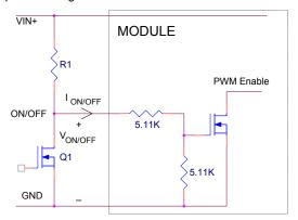
Figure 24. Remote On/Off Implementation using ON/OFF.
