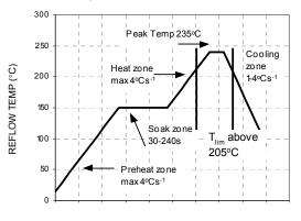
Figure 32. Reflow Profile for Tin/Lead (Sn/Pb) process.
