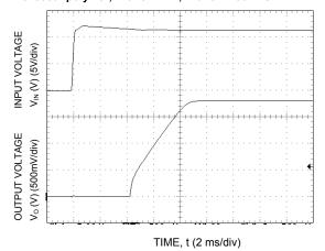
Figure 18. Typical Start-up Using Input Voltage ( $V_{IN} = 12V$ ,  $I_0 = I_{0,max}$ ).
