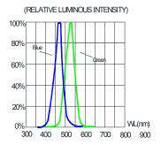
FIG.4 RELATIVE LUMINOUS INTENSITY VS. WAVELENGTH.
