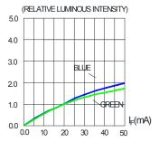
FIG.2 RELATIVE LUMINOUS INTENSITY VS. FORWARD CURRENT
