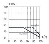
FIG.5 Green MAXIMUM FORWARD DC CURRENT VS AMBIENT TEMPERATURE (Tjmax=110°C)
