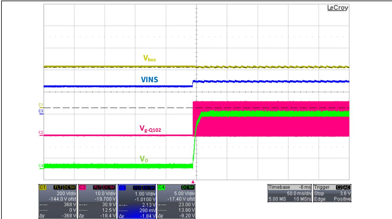
Figure 22 IC starts operation when  $V_{bus}$  resumes to normal value  $V_{bus-on} = 368 \text{ V}_{\text{DC}}$
