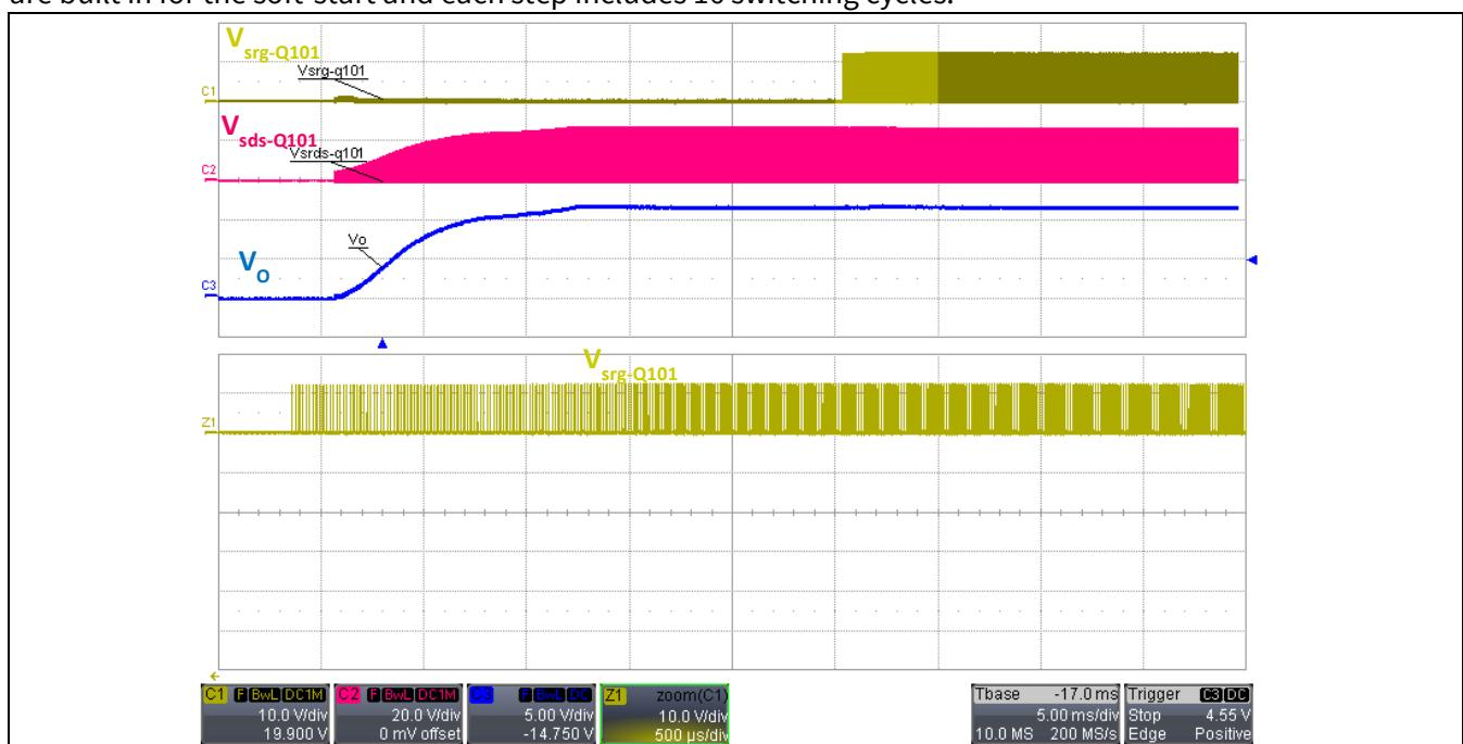
Figure 17 SR soft start at full load
