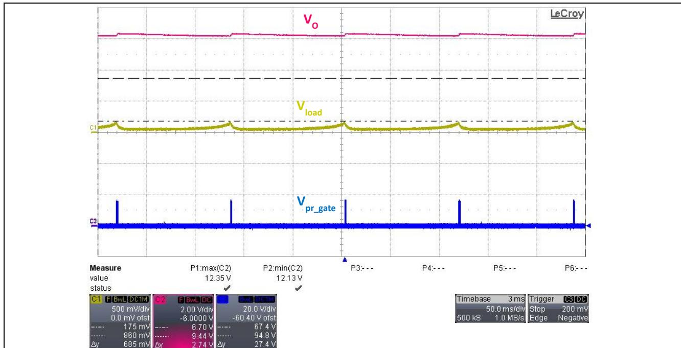
Figure 16 Burst mode operation at no load
