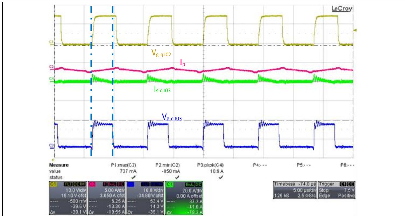
Figure 19 SR Driver on-time at light load
