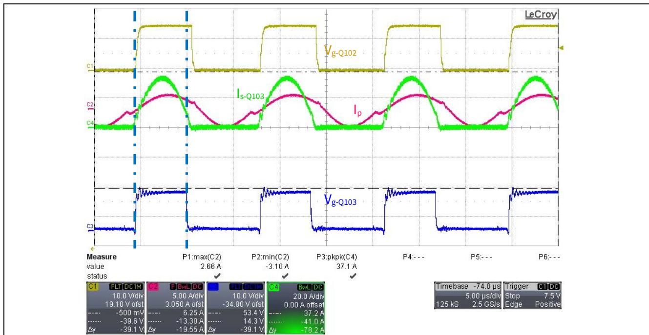
Figure 18 SR Driver on-time at Full load
