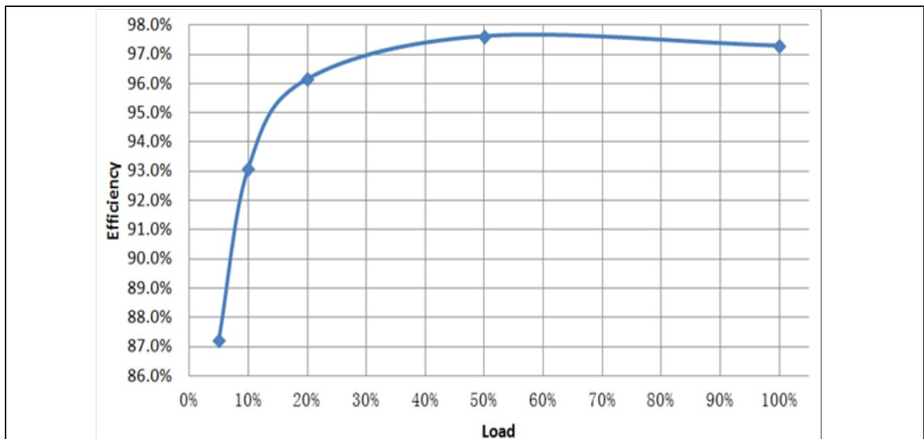
**Figure 13 LLC stage efficiency**
