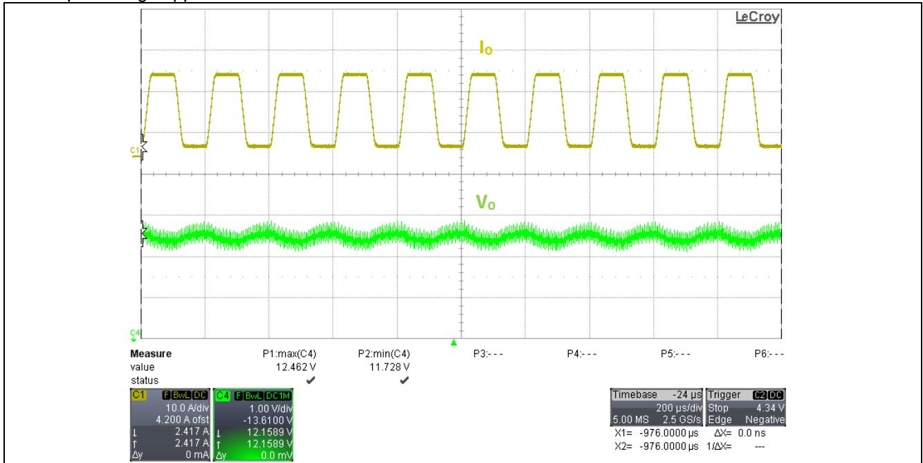
Figure 24 Dynamic load - 12 V @ 2.5 A ~ 20 A, 5 kHz, 800 mA/μs
