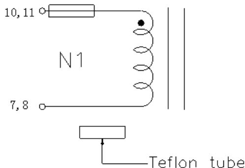
**Figure 10 LLC resonant transformer electrical diagram**
