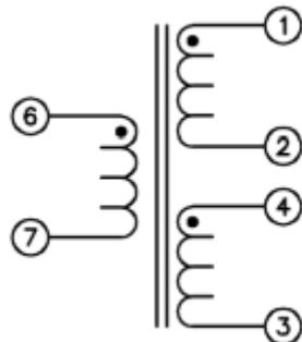
Figure 11 Pulse Transformer electrical diagram
