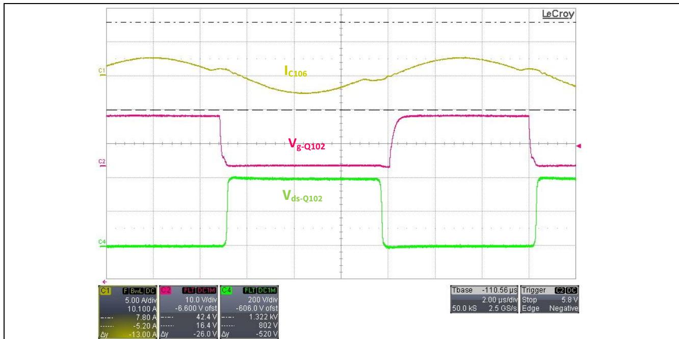
Figure 20 Zero voltage switching at full load
