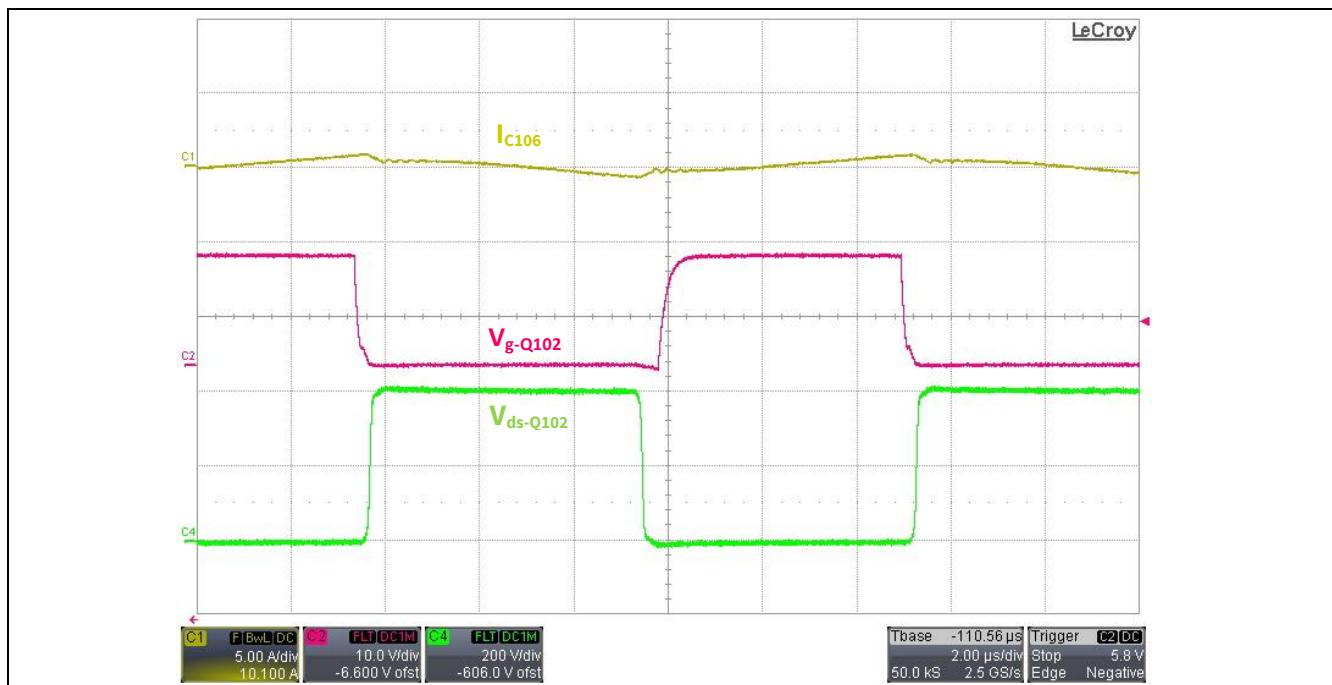
Figure 21 Zero voltage switching at full load
