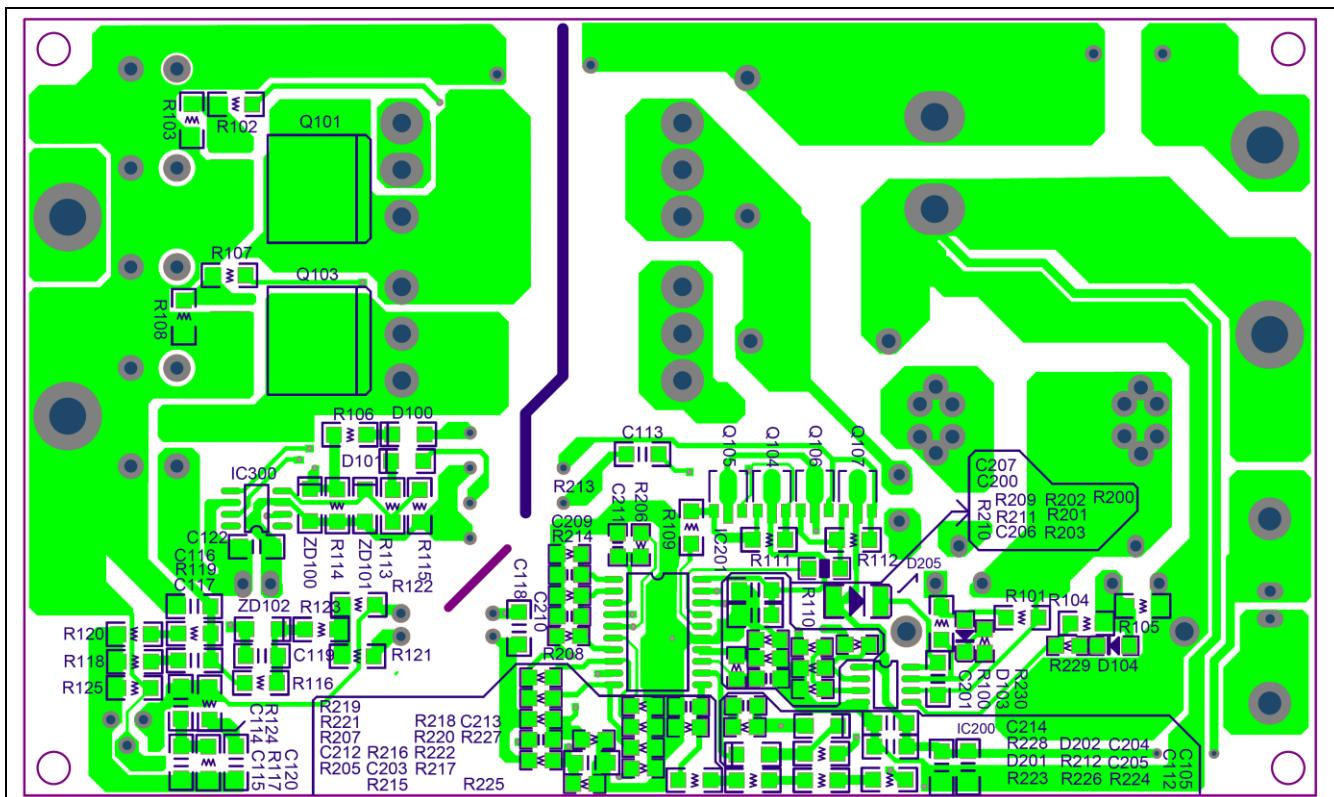
Figure 6 Solder side copper – View from solder side
