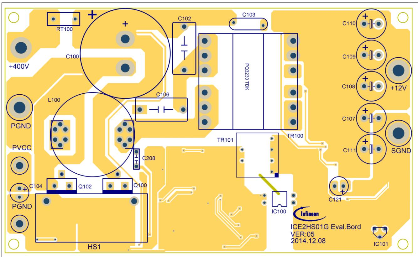
Figure 5 Component side copper – View from component side
