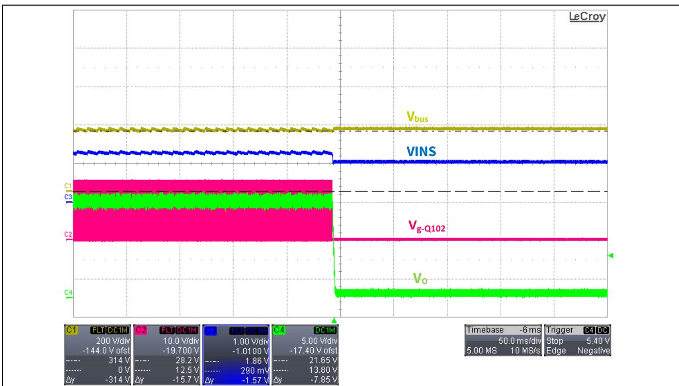
Figure 23 IC stop switching when  $V_{bus}$  drops to designed value  $V_{bus-off} = 314 \text{ V}$
