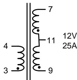
Figure 7 LLC resonant transformer electrical diagram
