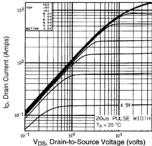
**Fig. 1 - Typical Output Characteristics,  $T_A = 25\text{ }^\circ\text{C}$**
