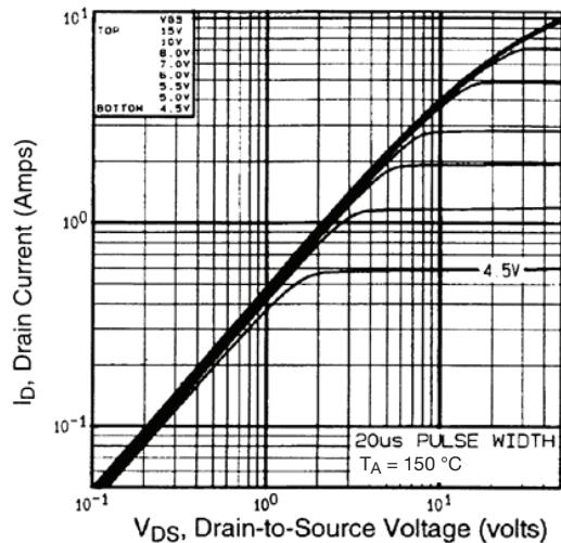
**Fig. 2 - Typical Output Characteristics,  $T_A = 150\text{ }^\circ\text{C}$**
