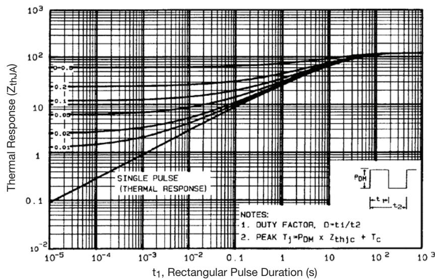
Fig. 11 - Maximum Effective Transient Thermal Impedance, Junction-to-Ambient
