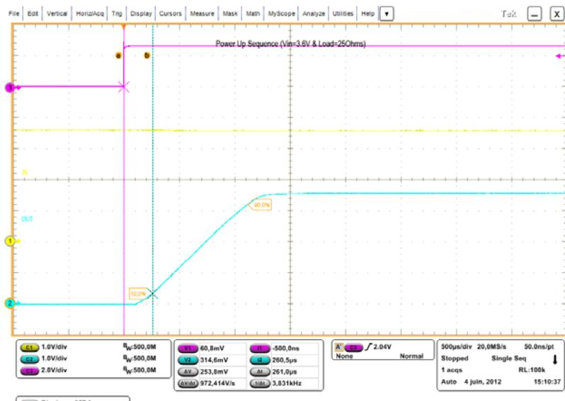
**Figure 12. Enable Time and Rise Time**
