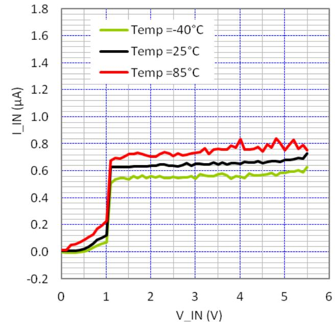
**Figure 11. Quiescent Current ( $\mu A$ ) vs. Temperature ( $^{\circ}C$ )**
