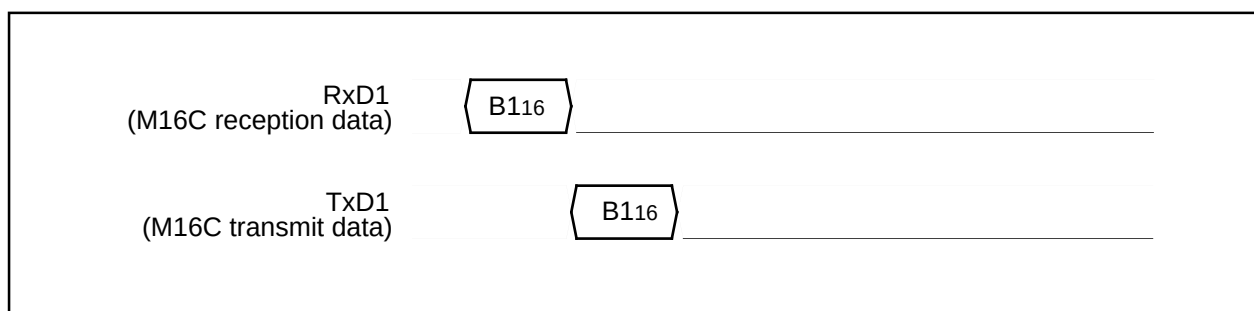
Figure 1.29.40. Timing of baud rate 19200
