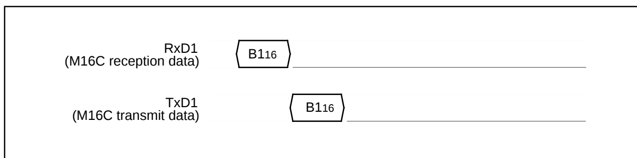
Figure 1.29.40. Timing of baud rate 19200
