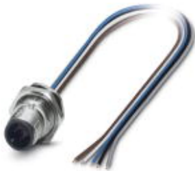
Sensor/actuator flush-type connector, 5-pos., M12 SPEEDCON, A-coded, rear/screw mounting with Pg9 thread, with 0.5 m TPE litz wire, 5 x 0.34 mm²
