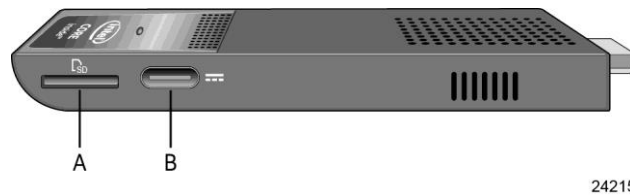
Figure 1. Left-Side View of Intel Compute Stick
