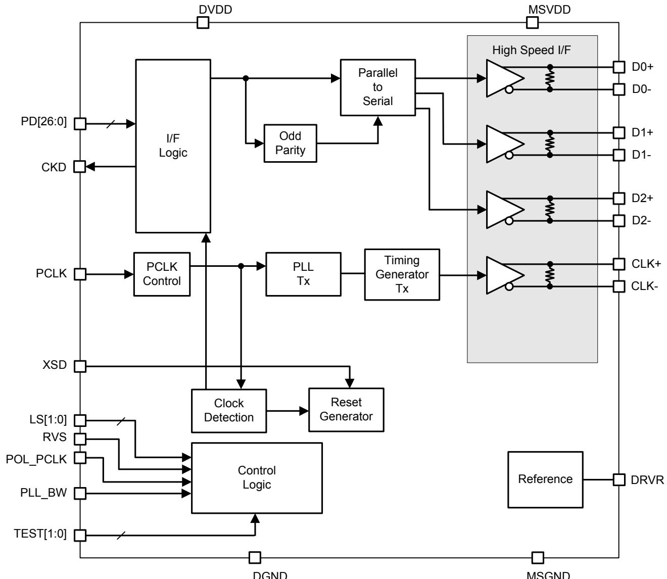
Fig.2. Block Diagram
