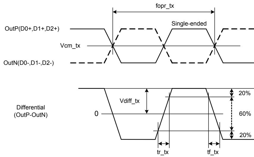
Fig.15. High-Speed Channel Electrical Characteristics
