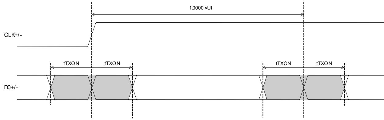
$$\begin{aligned} \text{UI} &= (1 \text{ cycle time of CLK+/-}) / 30 \\ N &= \text{Bit position } (0 \leq N \leq 30) \end{aligned}$$
