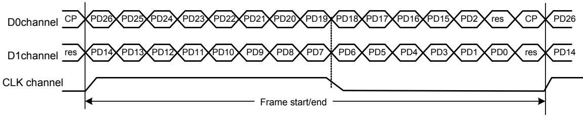
Fig.8. MSDL3 Protocol for 2-channel Data (27-bit)
