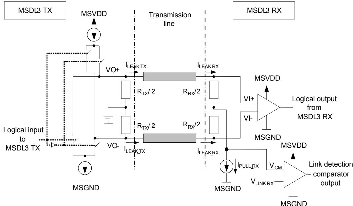
Fig.16. high-speed channel equivalent schematic.
