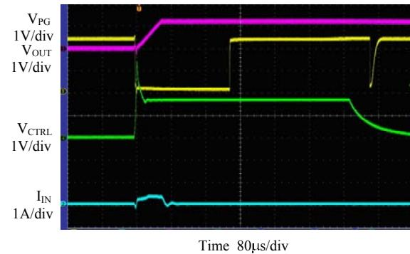
Figure 17.  $V_{CTRL}$  Start up and Shut down Waveform
