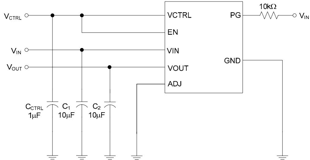
Figure 21. Typical Application of AP2132B for Fixed Version
