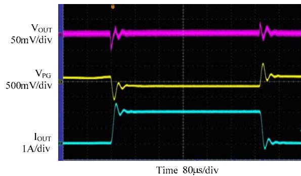
Figure 18. Load Transient
