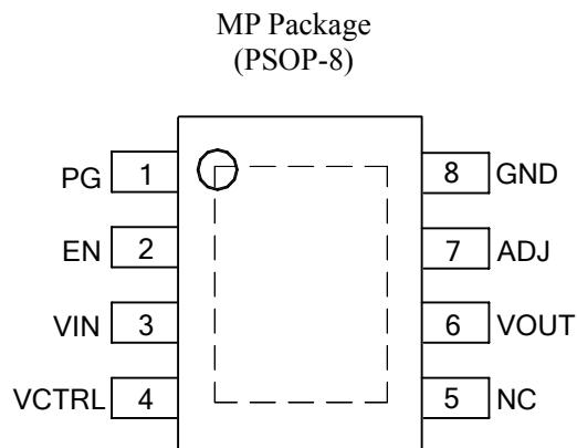
Figure 2. Pin Configuration of AP2132B (Top View)
