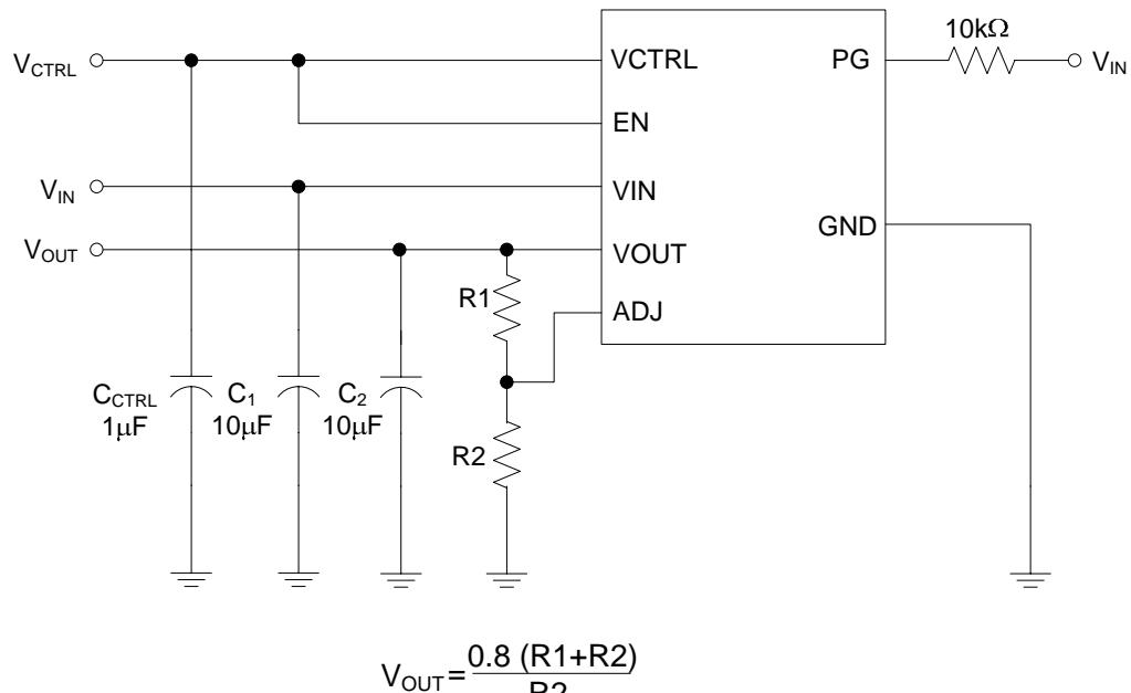
Figure 20. Typical Application of AP2132B for Adjustable Version
