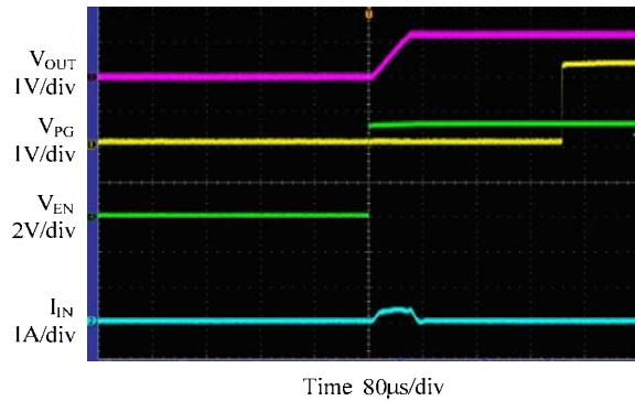
Figure 16.  $V_{EN}$  Start up Waveform
