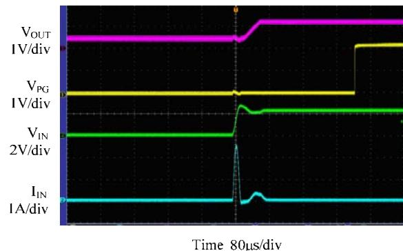
Figure 15.  $V_{IN}$  Start up Waveform
