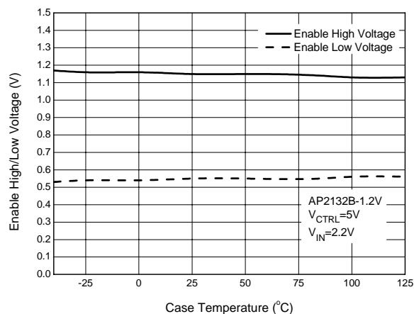
Figure 6. Enable High/Low Voltage vs. Case Temperature
