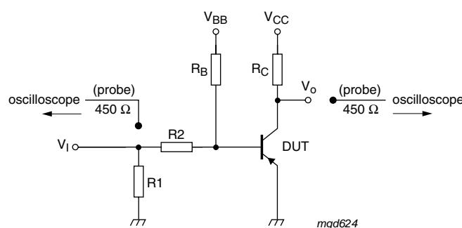
$V_{CC} = -10 \text{ V}$ ;  $I_C = -0.5 \text{ A}$ ;  $I_{Bon} = -0.025 \text{ A}$ ;  $I_{Boff} = 0.025 \text{ A}$
