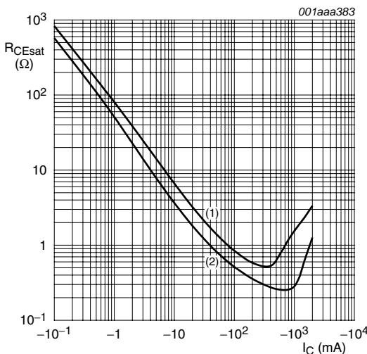
$T_{amb} = 25^\circ\text{C}$ (1)  $I_C/I_B = 50$ (2)  $I_C/I_B = 20$ **Fig 12. Collector-emitter saturation resistance as a function of collector current; typical values**
