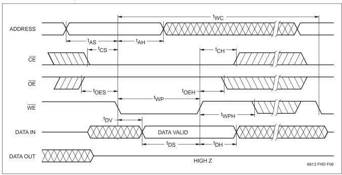
**Notes:** (4) t<sub>WC</sub> is the minimum cycle time to be allowed from the system perspective unless polling techniques are used. It is the maximum time the device requires to complete internal write operation.
