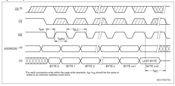
Notes: (5) Between successive byte writes within a page write operation,  $\overline{\text{OE}}$  can be strobed LOW: e.g. this can be done with  $\overline{\text{CE}}$  and  $\overline{\text{WE}}$  HIGH to fetch data from another memory device within the system for the next write; or with  $\overline{\text{WE}}$  HIGH and  $\overline{\text{CE}}$  LOW effectively performing a polling operation.
