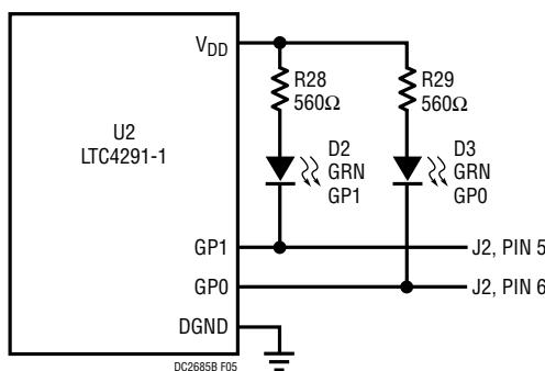
Figure 5. DC2684A-B, LTC4291-1 General Purpose I/O LED Indicators
