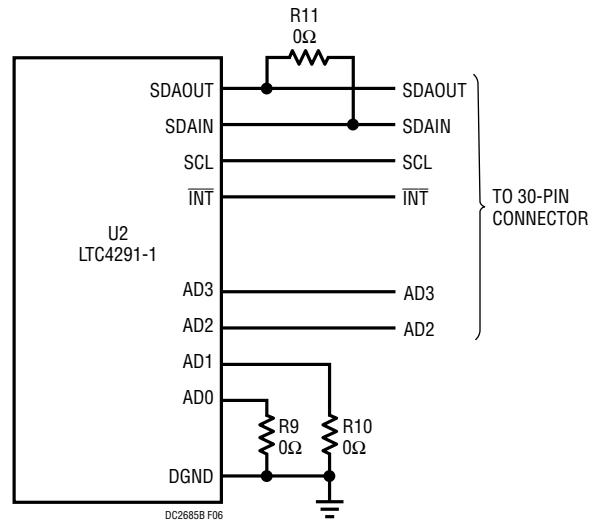
Figure 6. DC2684A-B, LTC4291-1 I<sup>2</sup>C and Address Connections
