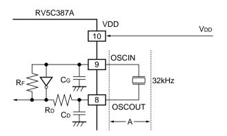
Typical externally-equipped element X'tal: 32.768kHz (R1= $30k\Omega$  TYP.) (CL=6pF to 8pF)
