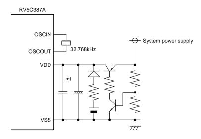
\*1) Install bypass capacitors for high-frequency and low-frequency applications in parallel in close vicinity to the RV5C387A.
