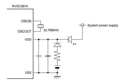
\*1) Connection in the example shown left may not affect the RV5C387A since it is designed to be operational even when the pin voltage exceeds VDD.
