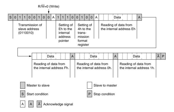
3) The third method to reading data from the internal register is to start reading immediately after writing to the slave address and the  $R/\overline{W}$  bit. Since the internal address pointer is set to Fh by default as described in 1), this method is only effective when reading is started from the internal address Fh.
