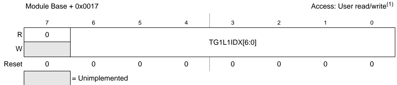
Figure 13-20. Trigger Generator 1 List 1 Index (TG1L1IDX)
