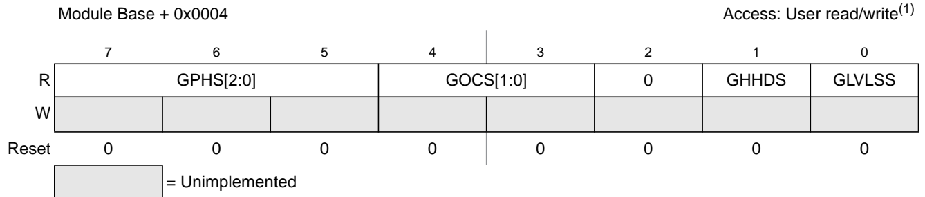
Figure 17-7. GDU Status Register (GDUSTAT)
