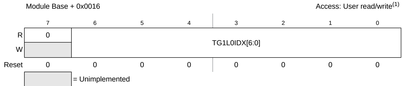
Figure 13-19. Trigger Generator 1 List 0 Index (TG1L0IDX)
