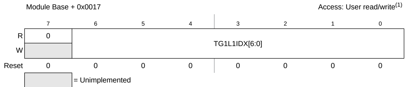
Figure 13-20. Trigger Generator 1 List 1 Index (TG1L1IDX)
