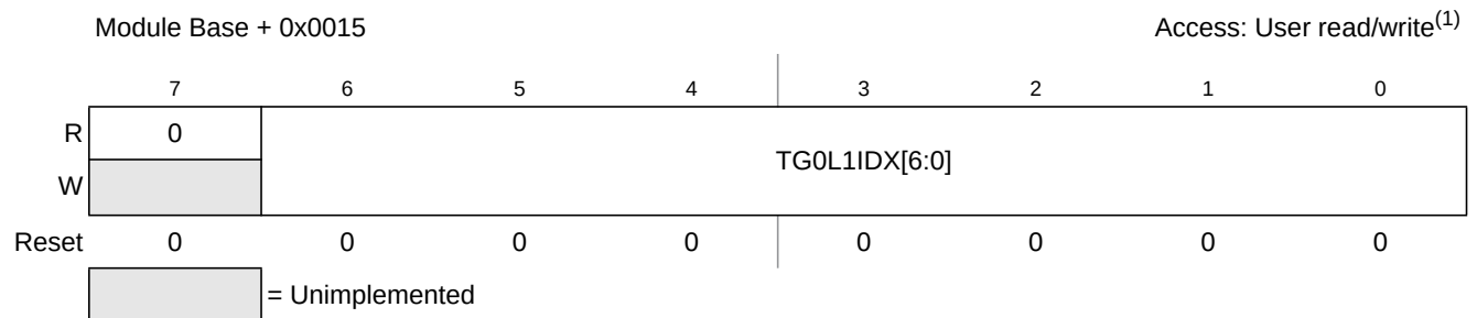
Figure 13-18. Trigger Generator 0 List 1 Index (TG0L1IDX)
