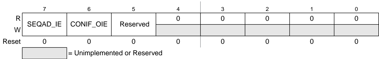
Figure 9-11. ADC Interrupt Enable Register (ADCIE)
