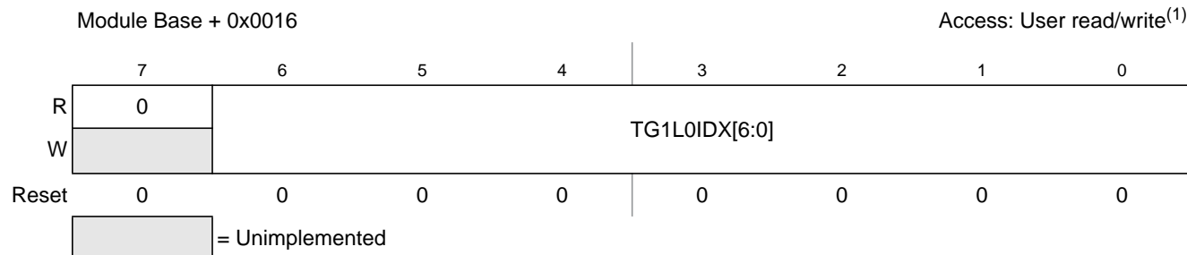
Figure 13-19. Trigger Generator 1 List 0 Index (TG1L0IDX)
