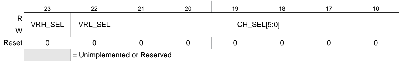
Figure 9-19. ADC Command Register 1 (ADCCMD_1)
