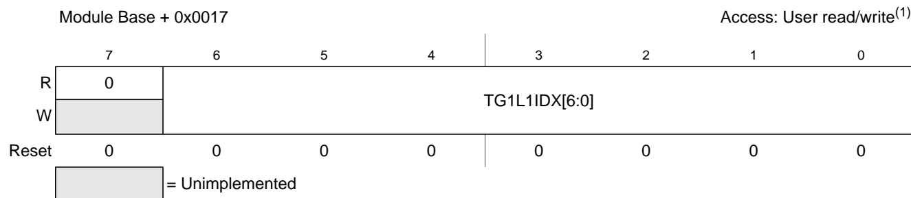
Figure 13-20. Trigger Generator 1 List 1 Index (TG1L1IDX)
