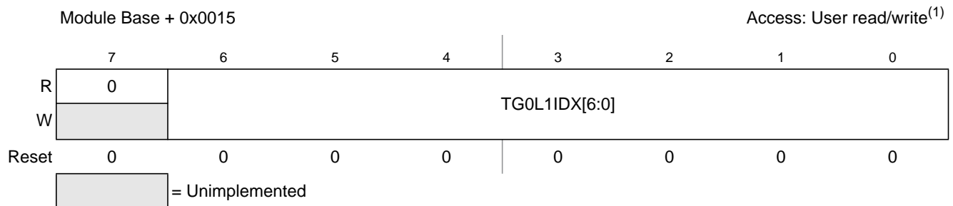
Figure 13-18. Trigger Generator 0 List 1 Index (TG0L1IDX)
