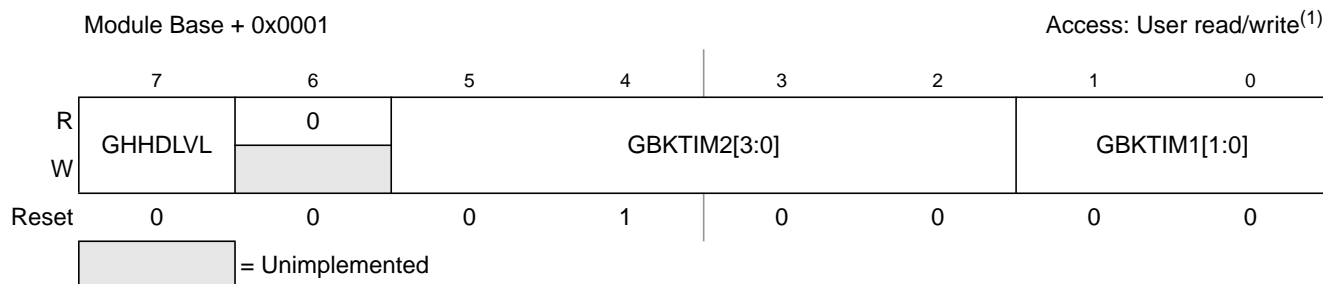
Figure 17-4. GDU Control Register (GDUCTR)
