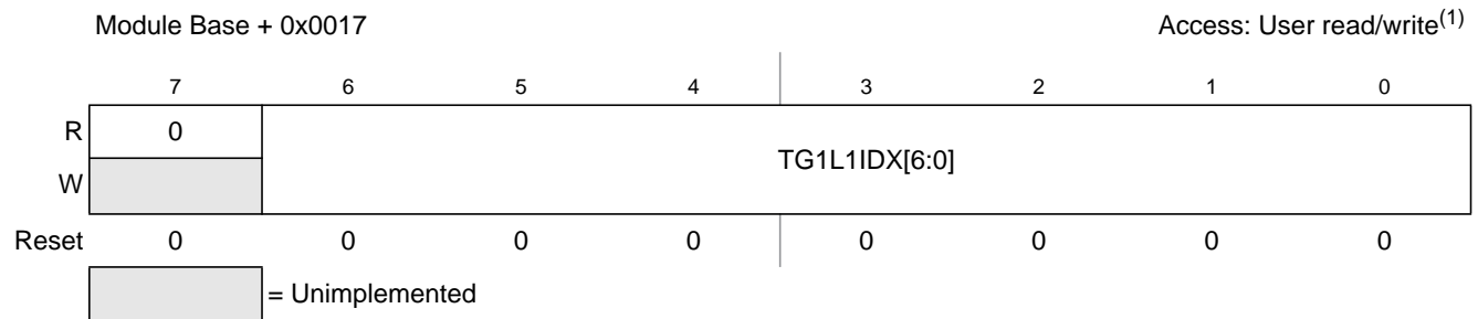
Figure 13-20. Trigger Generator 1 List 1 Index (TG1L1IDX)
