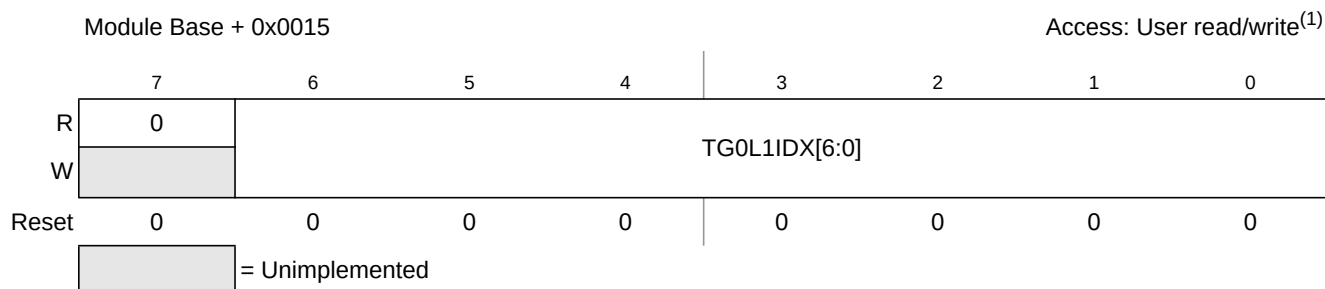
Figure 13-18. Trigger Generator 0 List 1 Index (TG0L1IDX)
