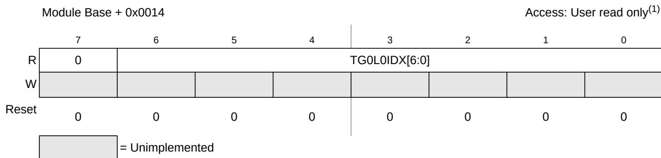
Figure 13-17. Trigger Generator 0 List 0 Index (TG0L0IDX)
