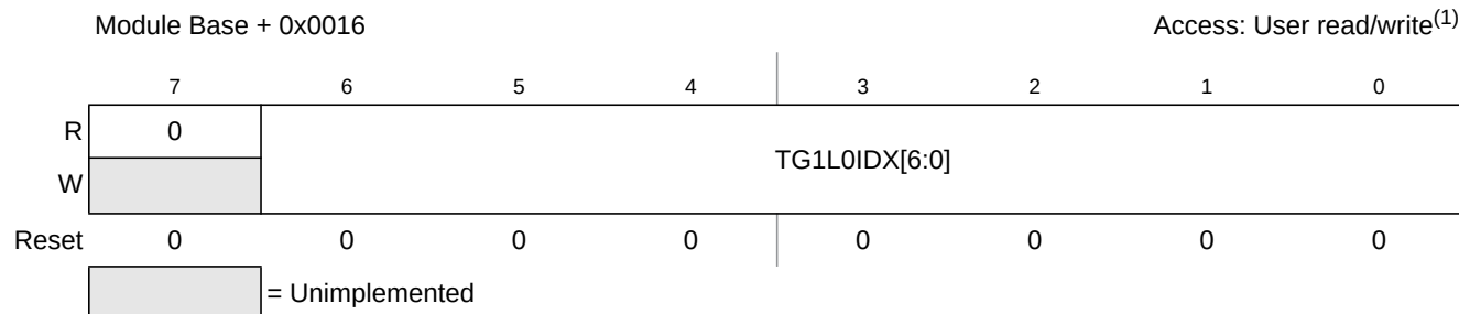
Figure 13-19. Trigger Generator 1 List 0 Index (TG1L0IDX)
