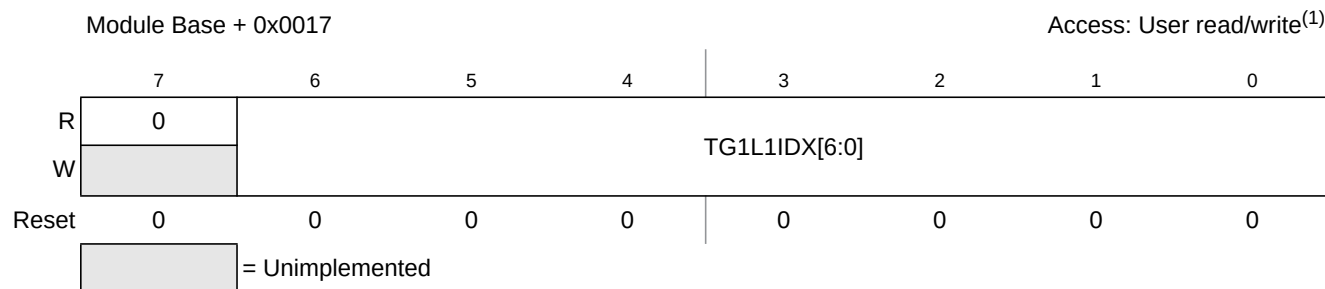
Figure 13-20. Trigger Generator 1 List 1 Index (TG1L1IDX)
