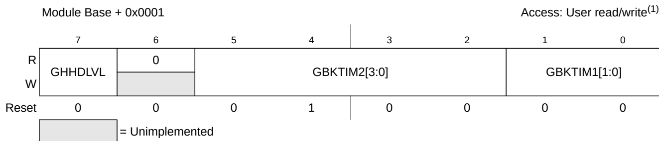
Figure 17-4. GDU Control Register (GDUCTR)
