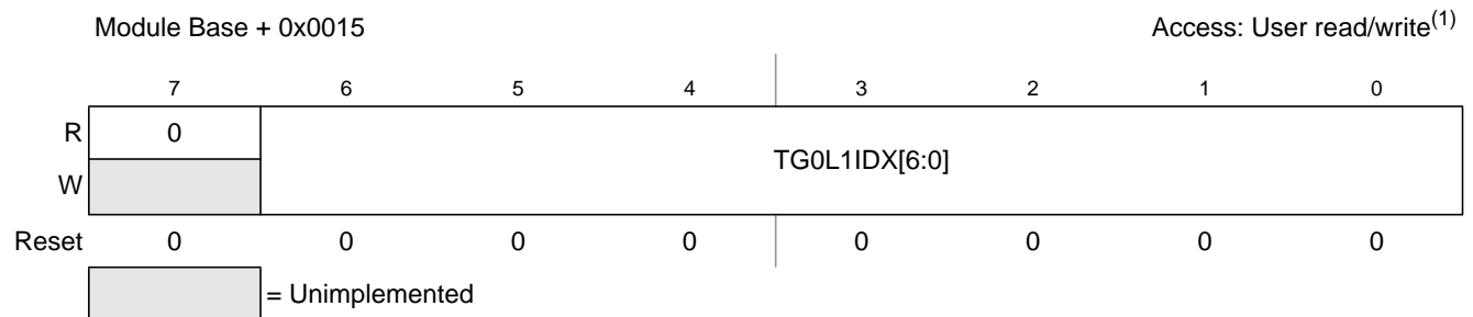
Figure 13-18. Trigger Generator 0 List 1 Index (TG0L1IDX)
