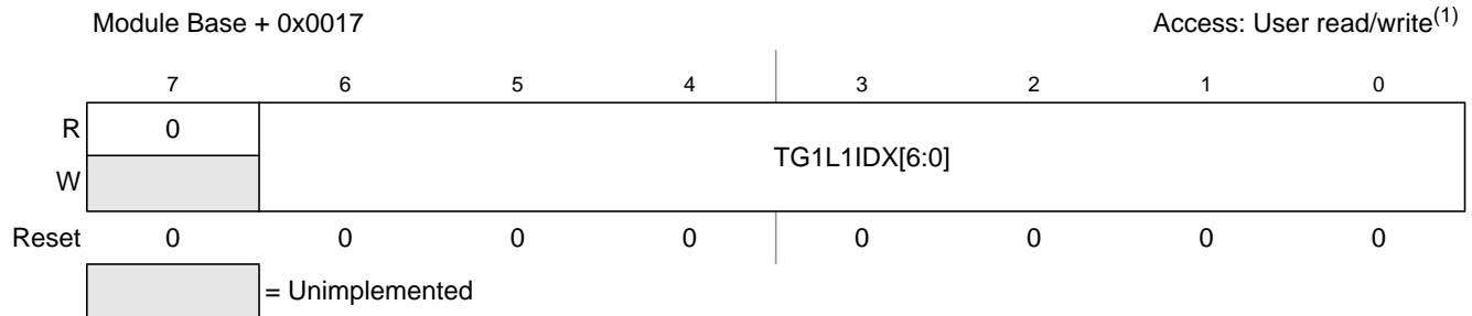
Figure 13-20. Trigger Generator 1 List 1 Index (TG1L1IDX)
