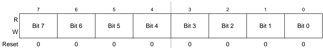
Figure 11-19. Timer Input Capture/Output Compare Register x Low (TCxL)
