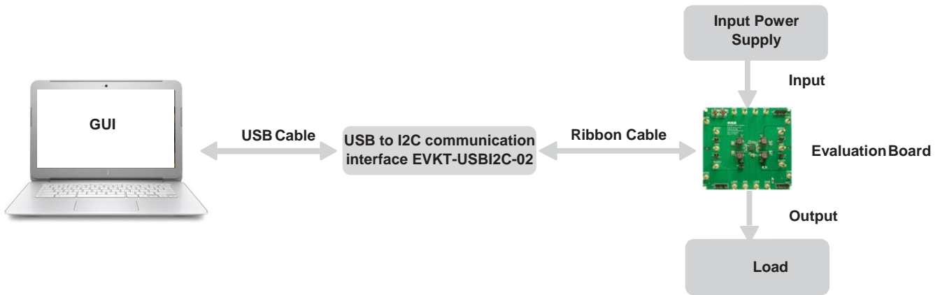
Figure 1: EVKT-5416 Evaluation Kit Set-Up
