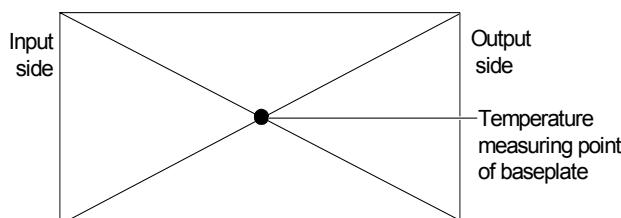
Figure 21 Temperature test point on base plate
