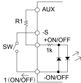
Figure 15 Connection of remote ON/OFF control (B)
