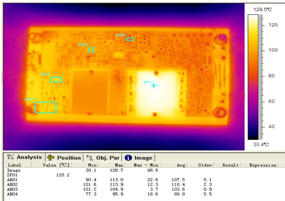
Figure 3 Thermal image,  $24\text{V}_{\text{in}}$ ,  $28\text{V}_{\text{o}}$ , full load, room temperature
