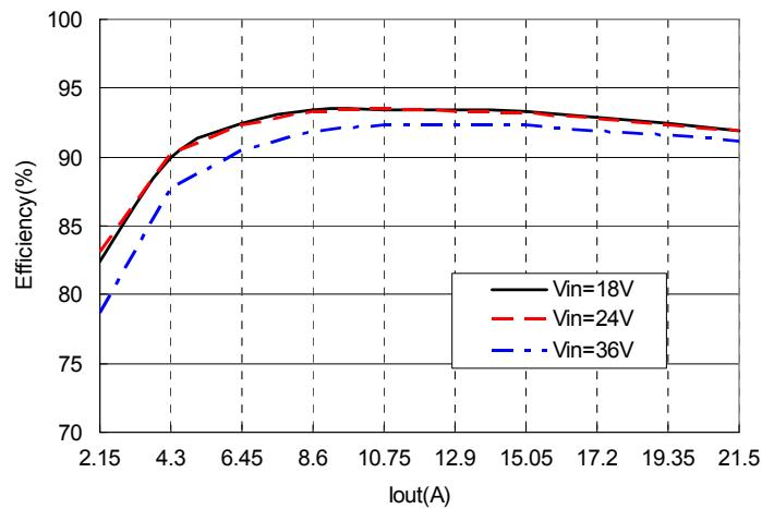
Figure 1 Efficiency vs. output current,  $T_a=25^\circ\text{C}$ ,  $V_o=28\text{V}$
