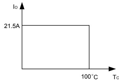
Figure 2 Output power derating curve
