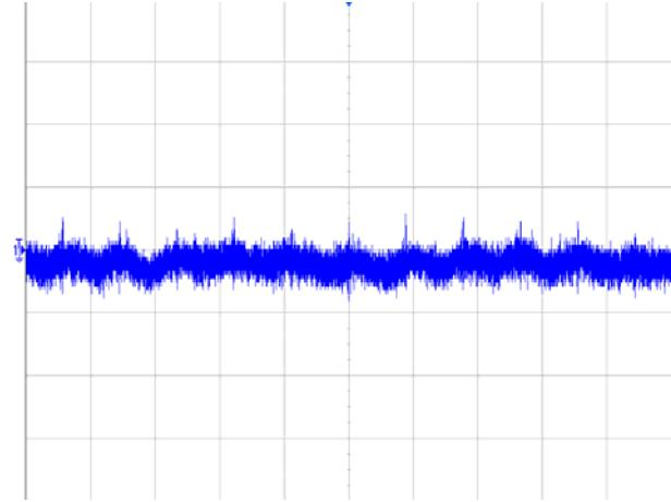
Figure 5 Input reflected ripple current (5 $\mu$ s/div, 20mA/div), see Figure 18 for test configuration
