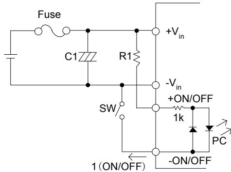
Figure 14 Connection of remote ON/OFF control (A)
