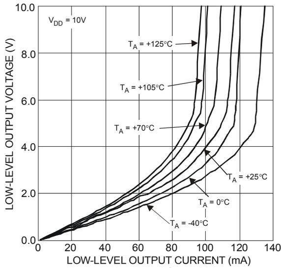
Figure 13 Low-Level Output Voltage vs. Low-Level Output Current
