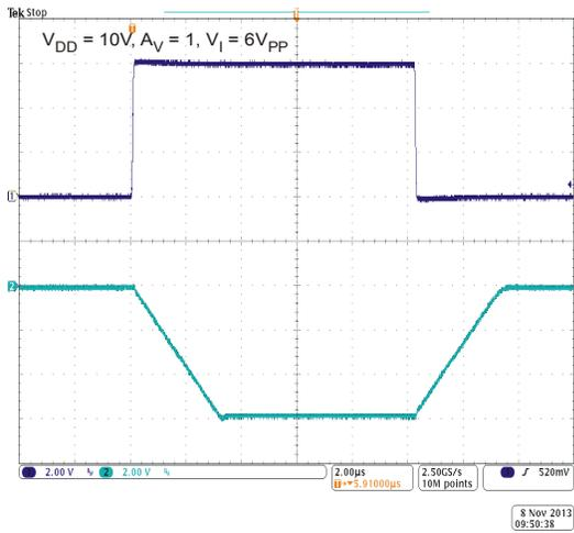
Figure 25 Inverting Large Signal Pulse Response  $V_{DD} = 10V$
