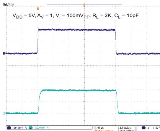
Figure 23 Voltage Follower Small Signal Pulse Response
