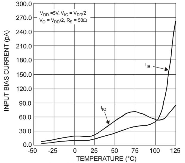
Figure 2 Input Bias and Offset Current vs. Temperature
