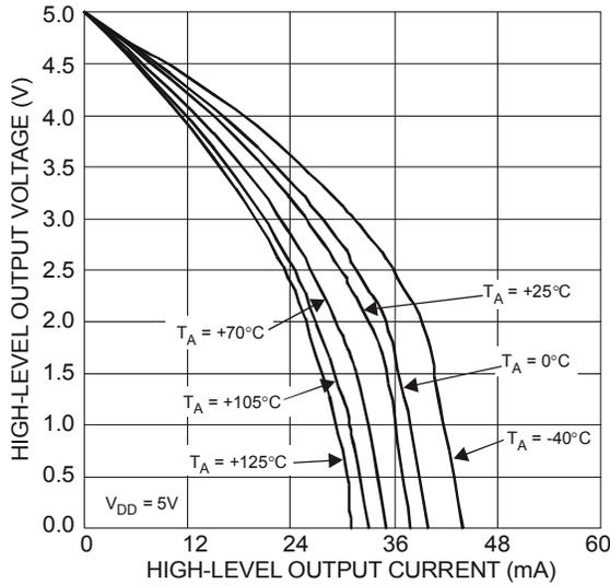
Figure 9 High-Level Output Voltage vs. High-Level Output Current
