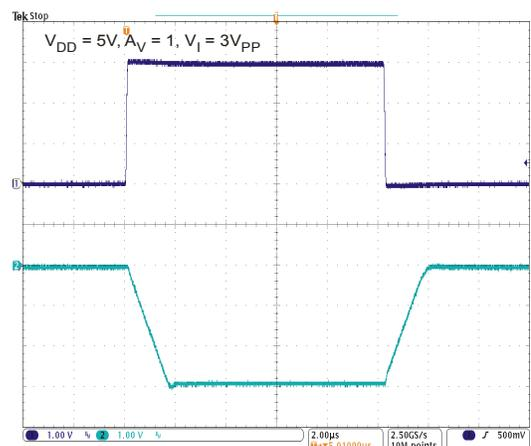
Figure 24 Inverting Large Signal Pulse Response  $V_{DD} = 5V$
