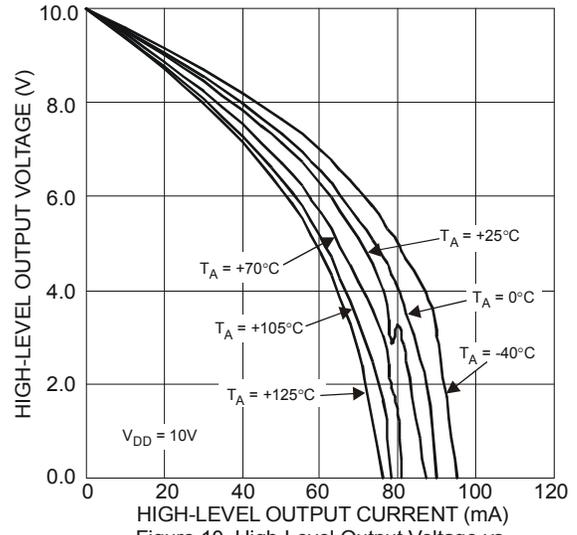
Figure 10 High-Level Output Voltage vs. High-Level Output Current
