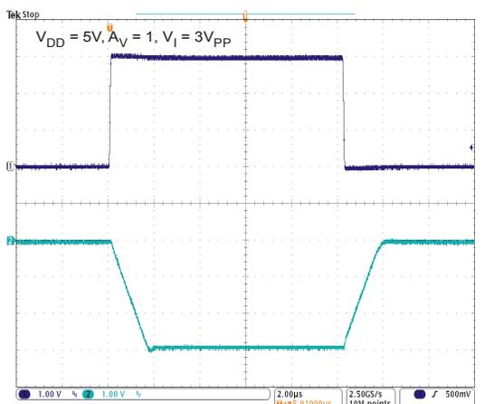
Figure 24 Inverting Large Signal Pulse Response  $V_{DD} = 5V$
