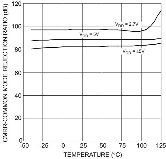
Figure 7 Common Mode Rejection Ratio vs. Temperature
