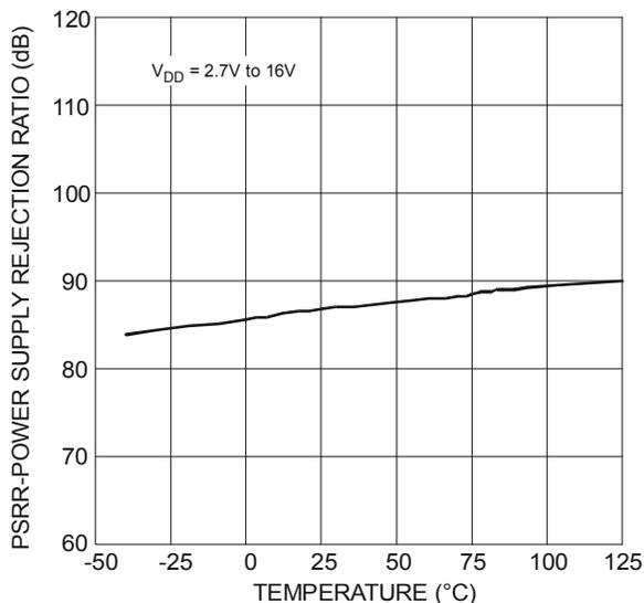
Figure 5 Power Supply Rejection Ratio vs. Temperature
