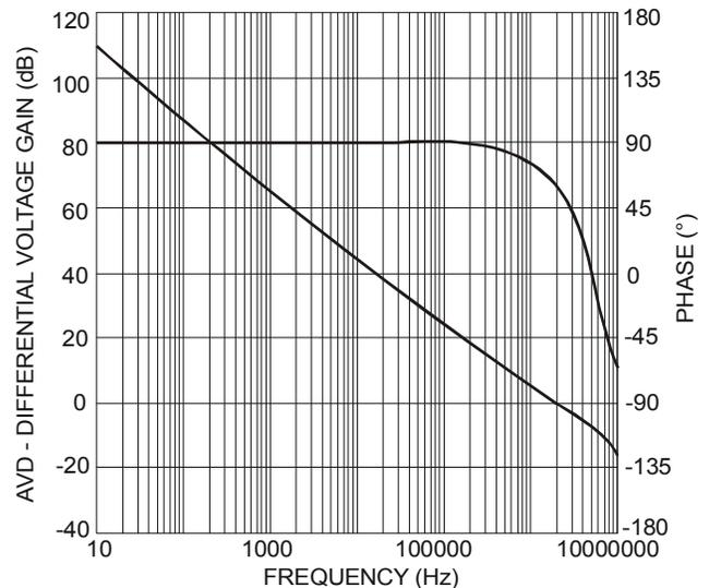
Figure 16 Differential Voltage Gain and Phase vs. Frequency
