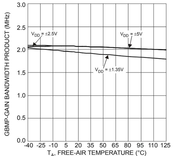
Figure 18 Gain Bandwidth Product vs. Free Air Temperature
