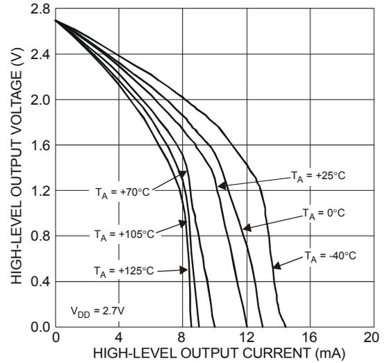
Figure 8 High-Level Output Voltage vs. High-Level Output Current
