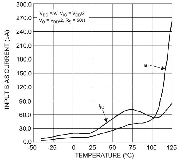
Figure 2 Input Bias and Offset Current vs. Temperature
