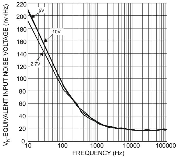
Figure 19 Equivalent Input Noise Voltage vs. Frequency
