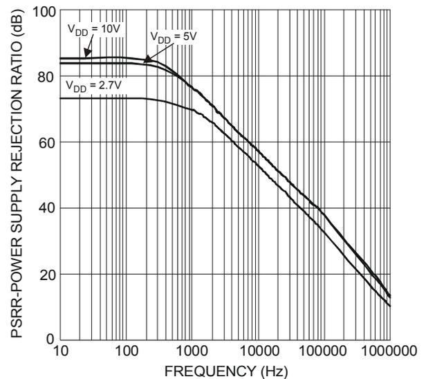
Figure 4 Power Supply Rejection Ratio vs. Frequency
