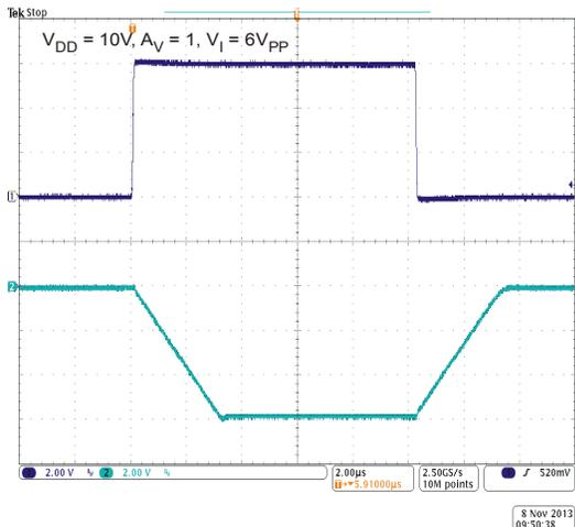
Figure 25 Inverting Large Signal Pulse Response  $V_{DD} = 10V$
