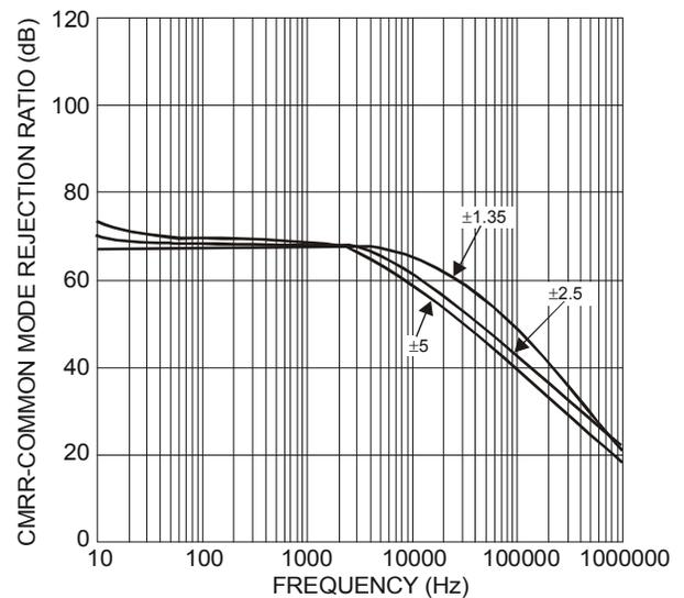
Figure 6 Common Mode Rejection Ratio vs. Frequency
