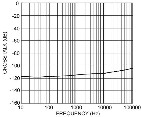
Figure 27 Crosstalk vs. Frequency TLV272
