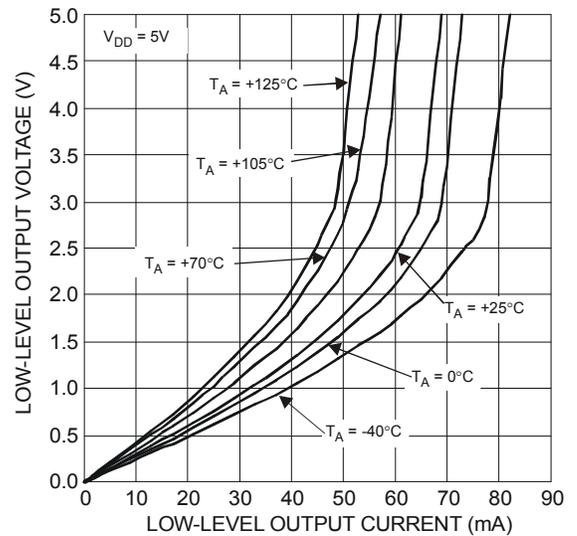
Figure 12 Low-Level Output Voltage vs. Low-Level Output Current
