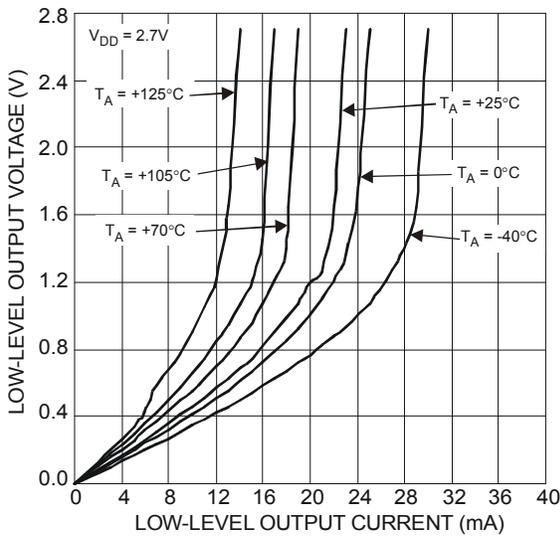
Figure 11 Low-Level Output Voltage vs. Low-Level Output Current
